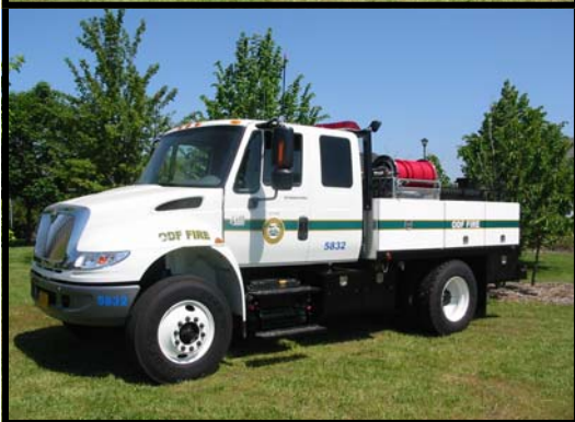
Engine 5832 650 gal. Type 3 engine Placed into service, June 2007. Built at the N. Cascade Shop.
