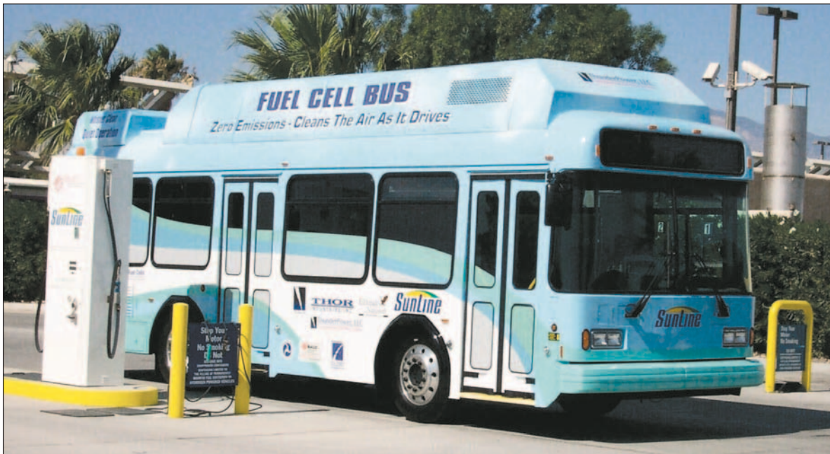
▲ Figure 5-1. Fuel cell-powered bus. Hydrogen fuel cell vehicles release no emissions in operations except water vapor.
