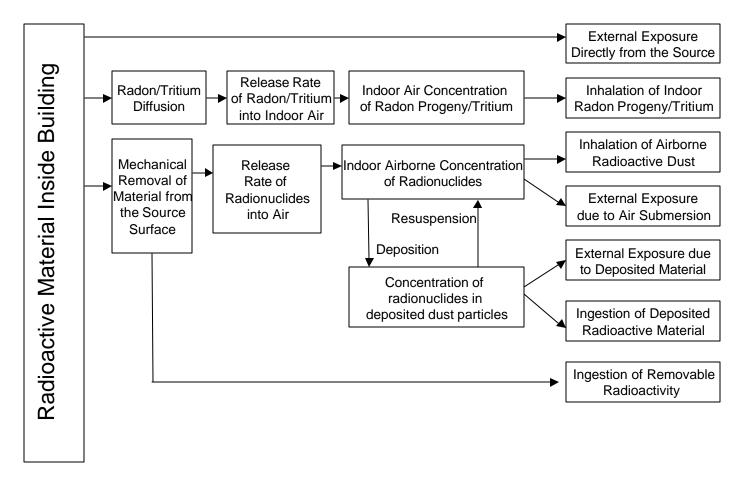
Figure 2.1 Exposure Pathways in the RESRAD-BUILD Code
