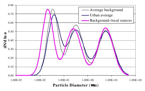
Figure 3.4 Trimodal Nature of Aerosol Particle Size Distribution
