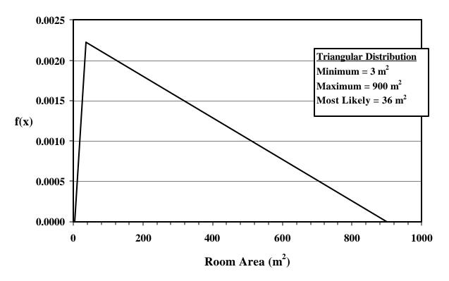
Figure A.3. Probability Density Function for Room Area
