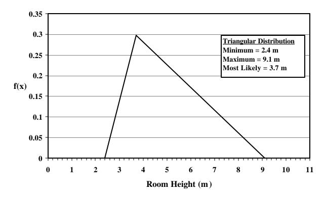
Figure A.4. Room Height Probability Density Function
