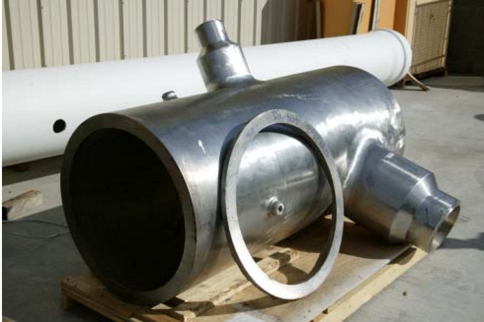
Figure 5.5 Large Blank Cast Spool Piece, Extracted from a Cancelled Spanish Nuclear Power Plant, Acquired by the EPRI NDE Center, and Loaned to PNNL for Advanced NDE Assessment Work
