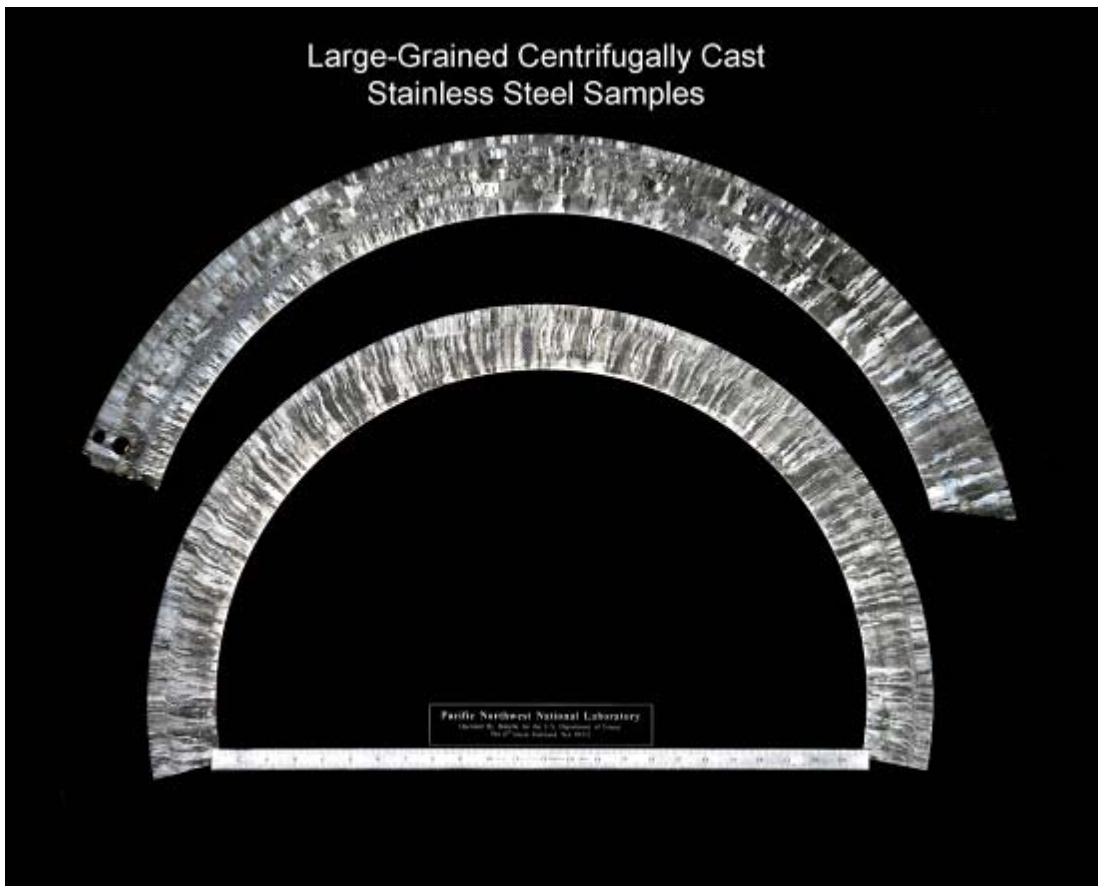
Figure A.28 Westinghouse and IHI Southwest Technologies Inc. Spool Pieces after Polishing and Etching
