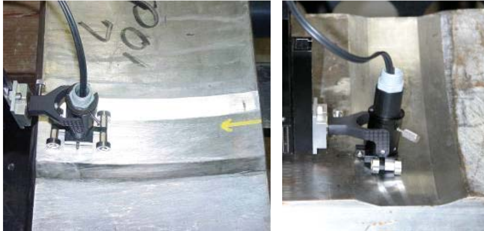
Figure 4.3 Top and Side Views of Inner Diameter Scan Configuration Using Eddy Current Testing Probe and Spring-Loaded Probe Sled for Translation over the Inner-Diameter Surface
