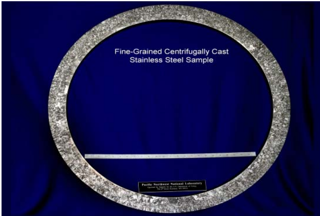
Figure A.25 EPRI NDE Center, Spanish Spool Piece Specimen, Polished and Etched Ring
