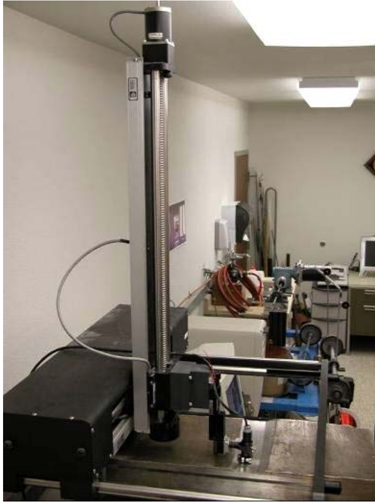
Figure 4.1 Automated x-y Eddy Current Testing Scanning System
