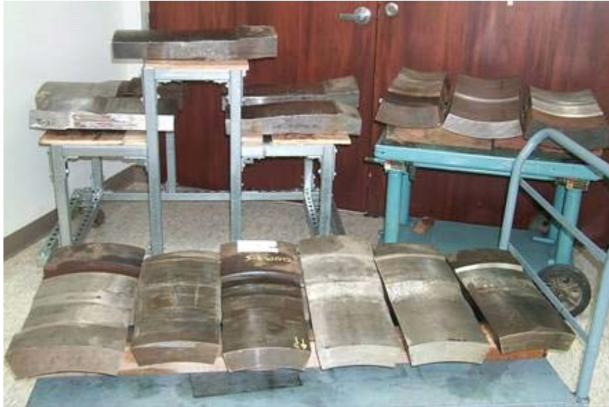
Figure 5.3 Westinghouse Owners Group Set of Cast Stainless Steel Specimens Used in This Study
