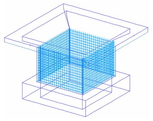
Figure 5-5 Shear Wall Rebars for Dynamic Simulation
