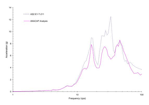
Figure 5-42 Comparison of Z-Direction Response between ANACAP Analysis at Upper Slab Corner No.2 and Measured Result for Run-3'
