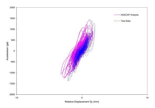
Figure 5-55 Comparison of Hysteresis Loops in Y-Direction for Run-4
