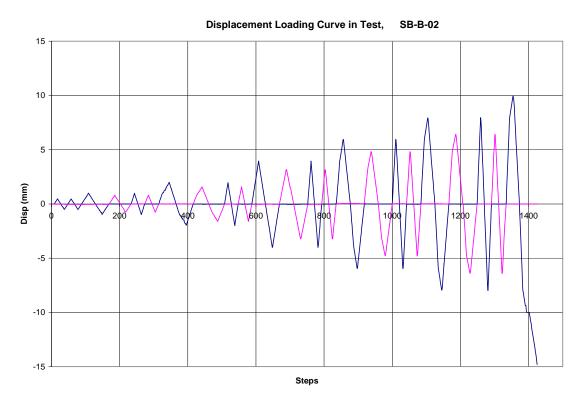
Figure 4-11 Displacement History at the Top of Shear Wall for SB-B-02
