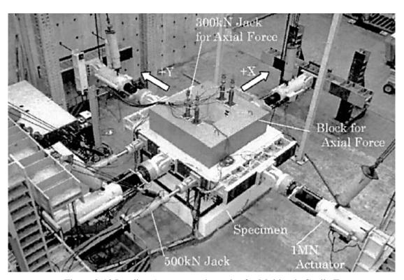
Figure 2-13 Loading Apparatus schematics for Multi-axis Cyclic Tests
