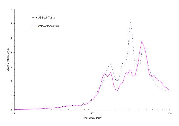
Figure 5-32 Comparison of Z-Direction Response between ANACAP Analysis at Upper Slab Corner No.1 and Measured Result for Run-3
