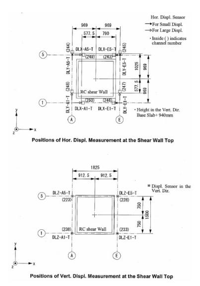
Figure 2-23 Schematic Locations of Displacement Gauges on Top of Walls
