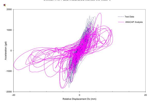
Figure 5-72 Comparison of Hysteresis Loops in X-Direction for Run-6
