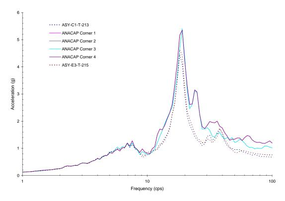
Figure 5-16 Comparison of Y-Direction Response between ANACAP Analysis at Upper Corners of Shear Walls and Measured Data for Run-2
