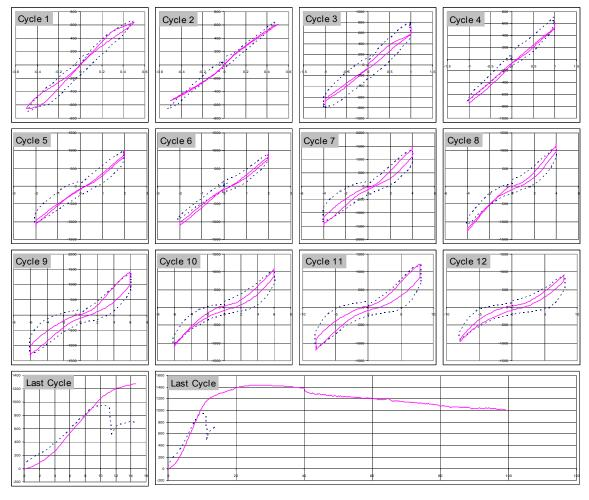
Figure 4-24 Cycle-By-Cycle Qx – Dx Relation For Rectangular Loading
