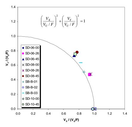
Figure 3-6 Maximum Vector Shear Forces Normalized by  $V_U/F$
