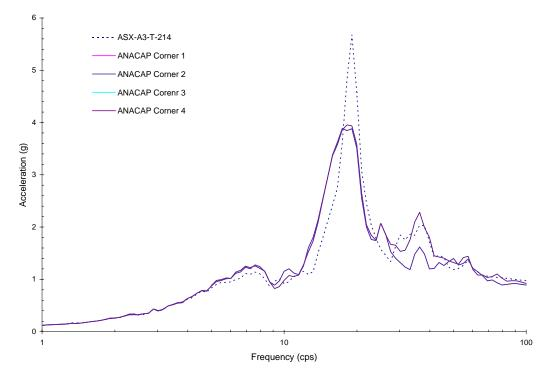
Figure 5-15 Comparison of X-Direction Response between ANACAP Analysis at Upper Corners of Shear Walls and Measured Data for Run-2
