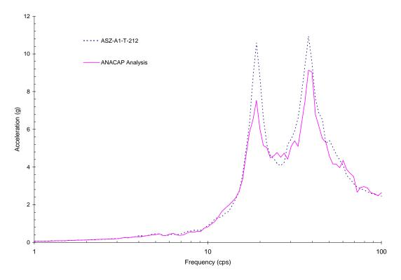
Figure 5-17 Comparison of Z-Direction Response between ANACAP Analysis at Upper Slab Corner No.1 and Measured Result for Run-2
