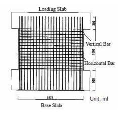
Figure 2-5 Reinforcement Arrangement for Box-Type Shear Wall Specimen
