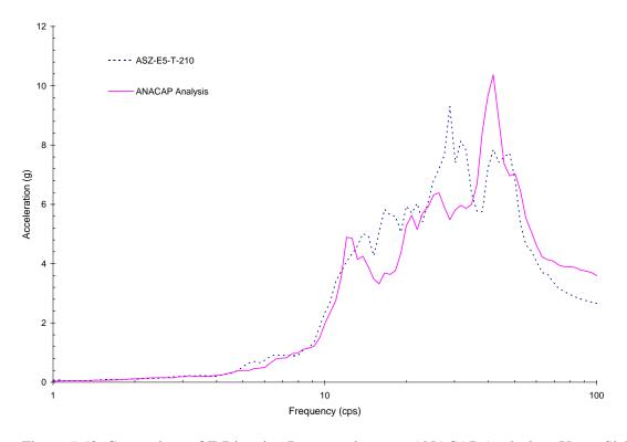
Figure 5-52 Comparison of Z-Direction Response between ANACAP Analysis at Upper Slab Corner No.3 and Measured Result for Run-4
