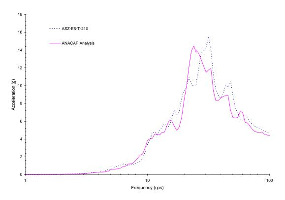
Figure 5-61 Comparison of Z-Direction Response between ANACAP Analysis at Upper Slab Corner No.3 and Measured Result for Run-5
