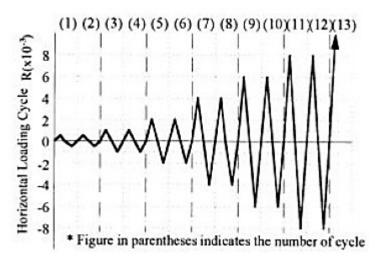
Figure 2-12 Loading Cycle Schematics for Uni-Directional Cyclic Tests
