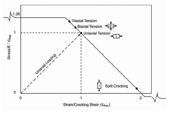
Figure 4-14 Criteria Curve for ANACAP Crack Initiation [from ANATECH 2004, Courtesy of ANATECH]
