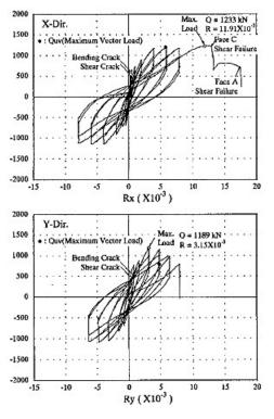
Figure 2-36 Shear-Deformation Hysteresis Loops for Specimen SB-C-01 (Rectangular Loading)
