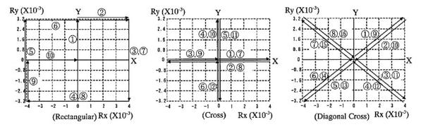
Figure 2-14 Loading Patterns for Multi-axis Cyclic Tests
