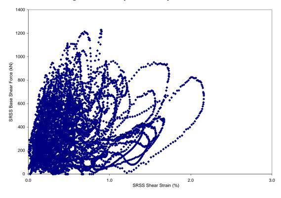
Figure 5-88 ANACAP Calculated SRSS Base Shear vs. SRSS Shear Strain Considering Prior Damages and X-Input Motion only for Run-6
