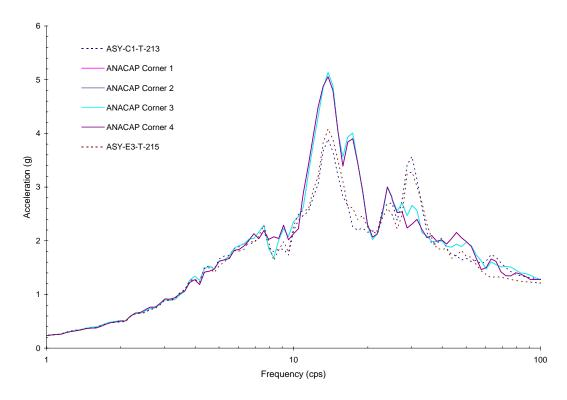
Figure 5-40 Comparison of Y-Direction Response between ANACAP Analysis at Upper Corners of Shear Walls and Measured Data for Run-3'
