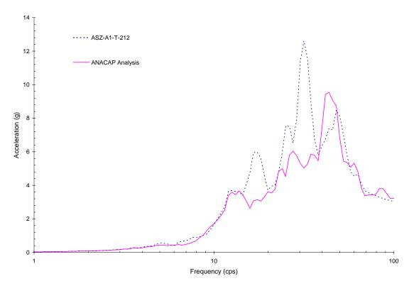
Figure 5-41 Comparison of Z-Direction Response between ANACAP Analysis at Upper Slab Corner No.1 and Measured Result for Run-3'
