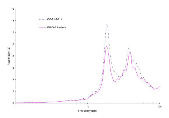
Figure 5-18 Comparison of Z-Direction Response between ANACAP Analysis at Upper Slab Corner No.2 and Measured Result for Run-2
