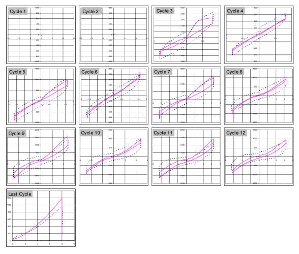
Figure 4-25 Cycle-By-Cycle Qy – Dy Relation For Rectangular Loading
