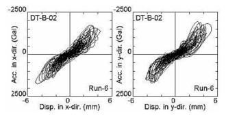
Figure 2-49 Horizontal Hysteresis Loops from Run 6 for DT-B-02
