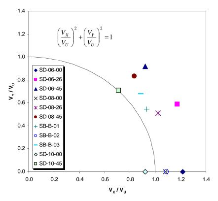
Figure 3-5 Maximum Vector Shear Forces Normalized by  $V_U$
