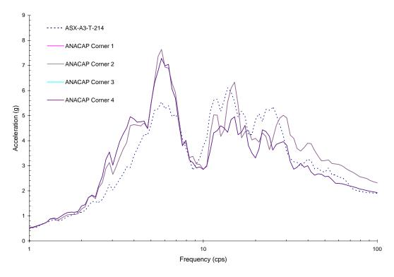
Figure 5-66 Comparison of X-Direction Response between ANACAP Analysis at Upper Corners of Shear Walls and Measured Data for Run-6
