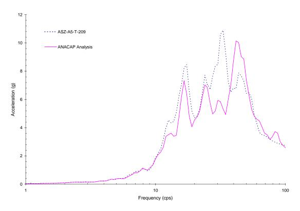
Figure 5-44 Comparison of Z-Direction Response between ANACAP Analysis at Upper Slab Corner No.4 and Measured Result for Run-3'
