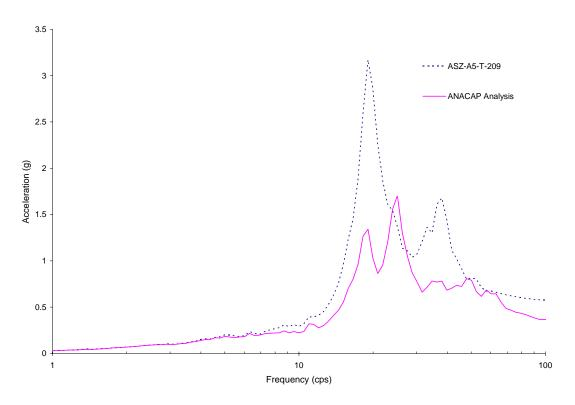
Figure 5-14 Comparison of Z-Direction Response between ANACAP Analysis at Upper Slab Corner No.4 and Measured Result for Run-1
