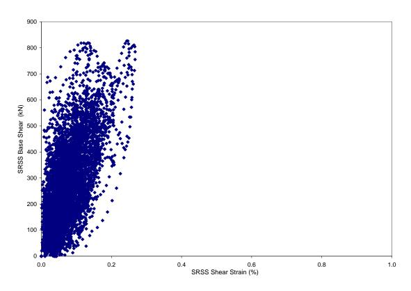
Figure 5-47 ANACAP Calculated SRSS Base Shear vs. SRSS Shear Strain for Run-3'
