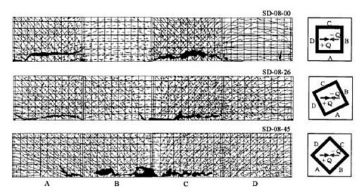
Figure 2-30 Crack Patterns of Shear Walls for SD-08 Series Specimens at Onset of Failure
