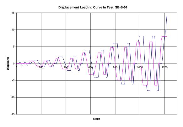
Figure 4-10 Displacement History at the Top of Shear Wall for SB-B-01
