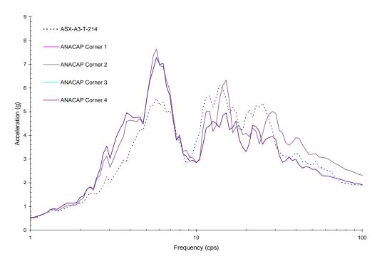
Figure 5-84 Comparison of X-Direction Response from ANACAP Analysis Considering Prior Damages but with X-Input Motion only and Test Result for Run-6
