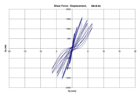
Figure 4-29 Qy – Dy Relation for Cross Loading
