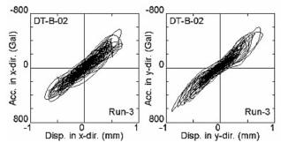
Figure 2-45 Horizontal Hysteresis Loops from Run 3 for DT-B-02
