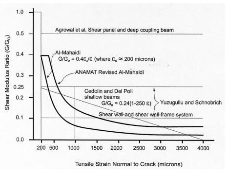
Figure 4-16 ANACAP Shear Retention Model [from Dunham R.S. and Rashid Y.R., 2003, Courtesy of ANATECH]
