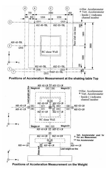
Figure 2-22 Schematic Locations of Accelerometers on Table Top and Top Weight
