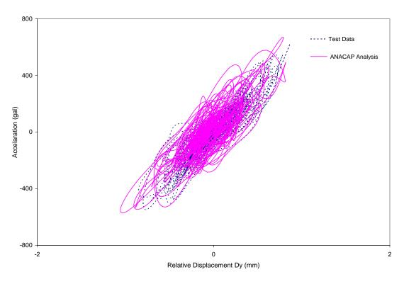
Figure 5-37 Comparison of Hysteresis Loops in Y-Direction for Run-3
