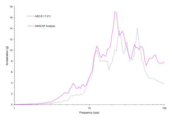
Figure 5-78 Comparison of ANACAP Analysis without Considering Prior Damages for Run-6 in Z-Direction at Upper Slab Corner No.2 and Measured Result
