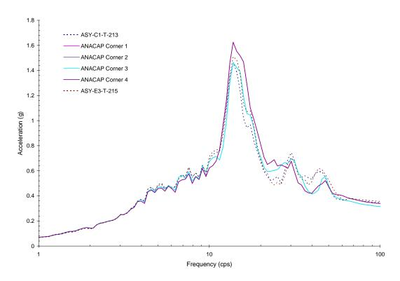
Figure 5-22 Comparison of Y-Direction Response between ANACAP Analysis at Upper Corners of Shear Walls and Measured Data for Run-2'
