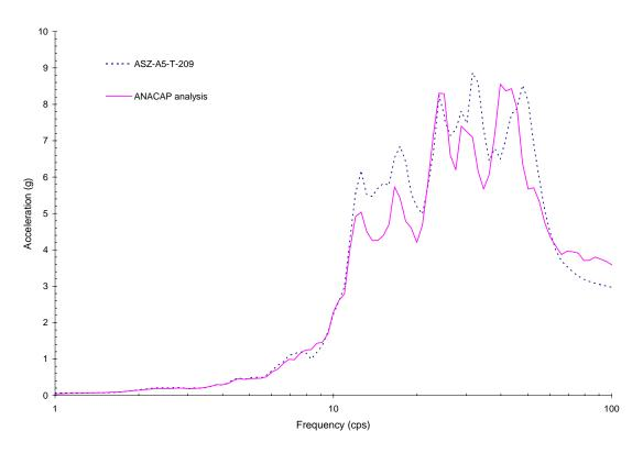
Figure 5-53 Comparison of Z-Direction Response between ANACAP Analysis at Upper Slab Corner No.4 and Measured Result for Run-4
