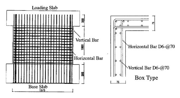
Figure 4-2 Rebar Configuration (Unit mm) [after Hiroshi, 2001]
