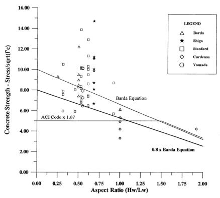
Figure 3-1 Concrete Shear Wall Strength as a Function of Aspect Ratio [from ASCE 43-05, 2004, With permission from ASCE]
