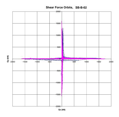
Figure 4-32 Shear Force Orbits for Cross Loading
