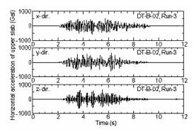
Figure 2-41 Three Orthogonal Components of Acceleration Response of Upper Slab for Specimen DT-B-02
