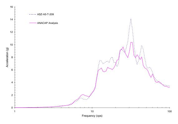
Figure 5-62 Comparison of Z-Direction Response between ANACAP Analysis at Upper Slab Corner No.4 and Measured Result for Run-5
