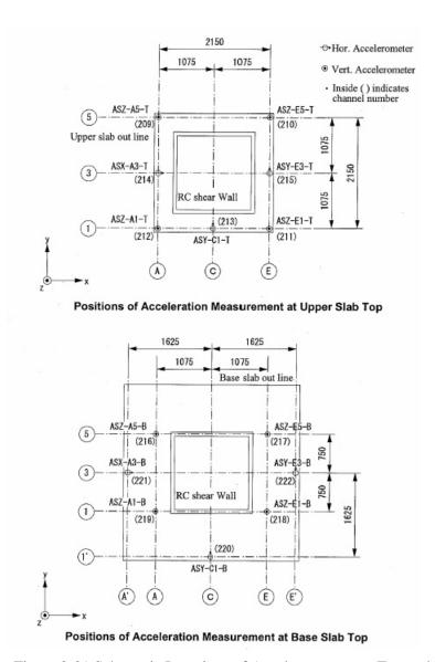
Figure 2-21 Schematic Locations of Accelerometers on Top and Base Slabs
