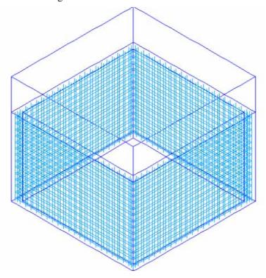
Figure 4-19 ANACAP Rebars Model for the Shear Wall
