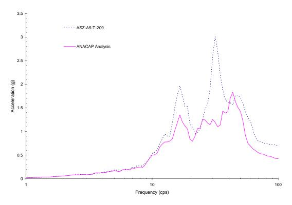
Figure 5-26 Comparison of Z-Direction Response between ANACAP Analysis at Upper Slab Corner No.4 and Measured Result for Run-2'
