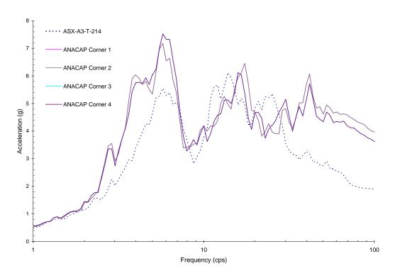
Figure 5-75 Comparison of ANACAP Analysis without Considering Prior Damages for Run-6 in X-Direction at Upper Corners of Shear Walls and Measured Data
