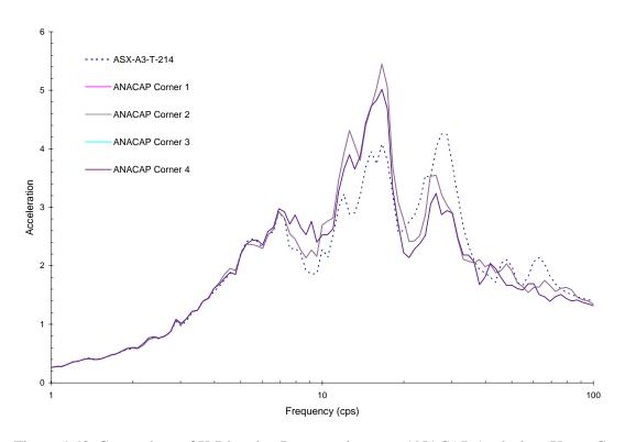
Figure 5-48 Comparison of X-Direction Response between ANACAP Analysis at Upper Corners of Shear Walls and Measured Data for Run-4
