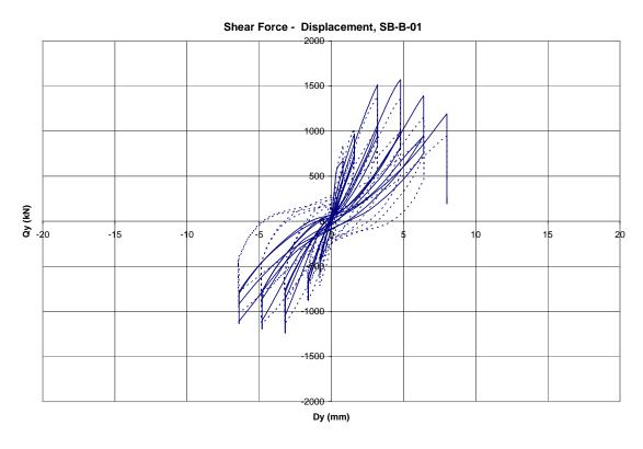
Figure 4-23 Qy - Dy Relation for Rectangular Loading
