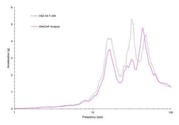
Figure 5-35 Comparison of Z-Direction Response between ANACAP Analysis at Upper Slab Corner No.4 and Measured Result for Run-3
