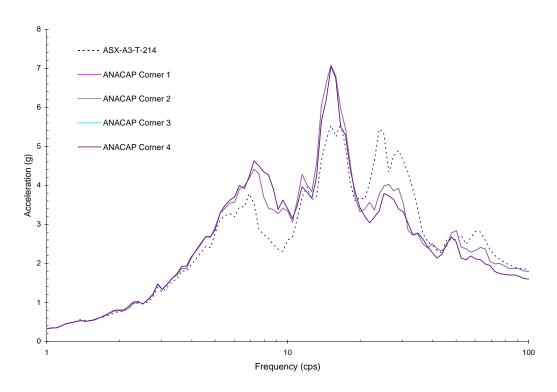
Figure 5-57 Comparison of X-Direction Response between ANACAP Analysis at Upper Corners of Shear Walls and Measured Data for Run-5
