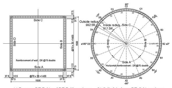
(a) Box-type DT-B-01 and DT-B-02 specimen  $\,$  (b) Cylindrical type DT-C-01 specimen
