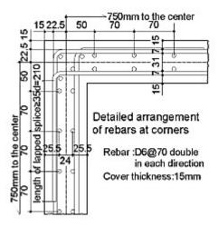
Figure 2-10 Rebar Details at Corners of Box-Type Specimens
