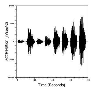
Figure 5-6 X-Input Motions for ANACAP Simulation Analysis
