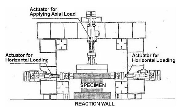
Figure 2-11 Loading Apparatus Schematics for Uni-Directional Cyclic Tests
