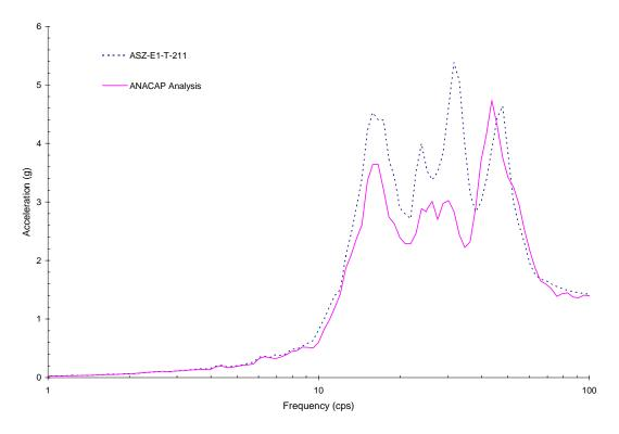
Figure 5-33 Comparison of Z-Direction Response between ANACAP Analysis at Upper Slab Corner No.2 and Measured Result for Run-3
