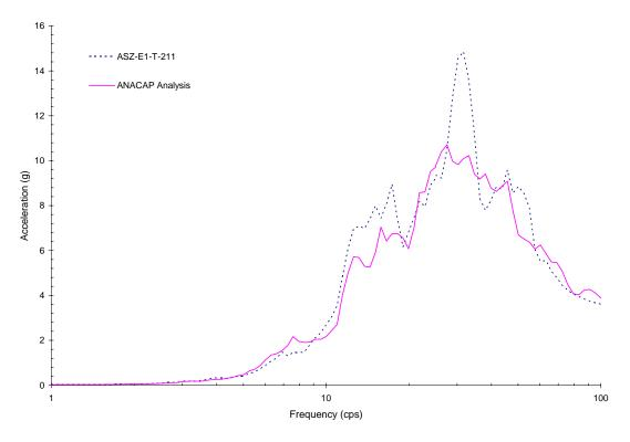
Figure 5-60 Comparison of Z-Direction Response between ANACAP Analysis at Upper Slab Corner No.2 and Measured Result for Run-5
