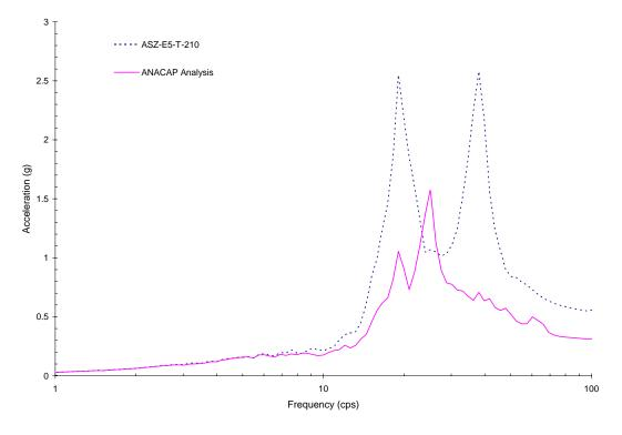
Figure 5-13 Comparison of Z-Direction Response between ANACAP Analysis at Upper Slab Corner No. 3 and Measured Result for Run-1
