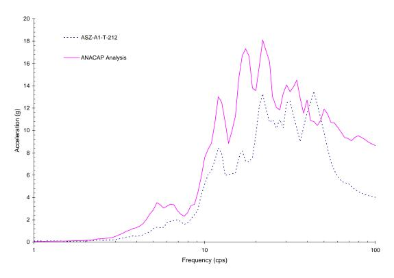
Figure 5-77 Comparison of ANACAP Analysis without Considering Prior Damages for Run-6 in Z-Direction at Upper Slab Corner No.1 and Measured Result
