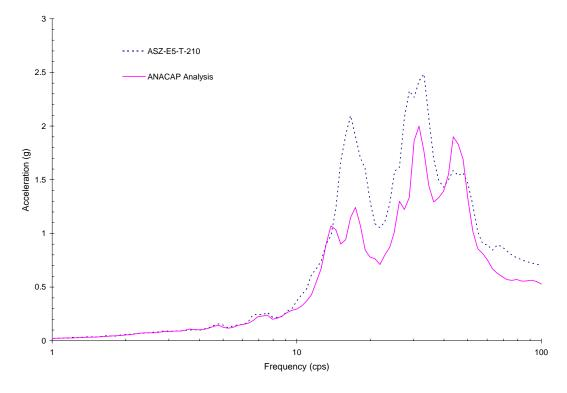
Figure 5-25 Comparison of Z-Direction Response between ANACAP Analysis at Upper Slab Corner No.3 and Measured Result for Run-2'
