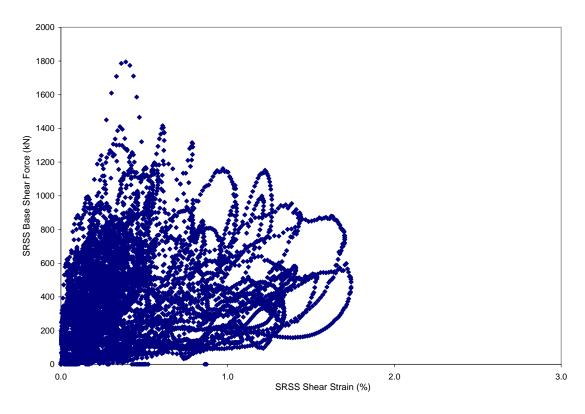
Figure 5-89 ANACAP Calculated SRSS Base Shear vs. SRSS Shear Strain Considering No Prior Damages and X-Input Motion only for Run-6
