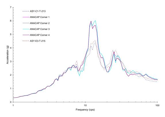
Figure 5-49 Comparison of Y-Direction Response between ANACAP Analysis at Upper Corners of Shear Walls and Measured Data for Run-4
