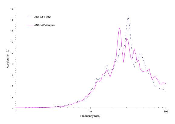
Figure 5-59 Comparison of Z-Direction Response between ANACAP Analysis at Upper Slab Corner No.1 and Measured Result for Run-5
