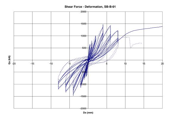
Figure 4-22 Qx – Dx Relation for Rectangular Loading
