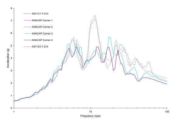
Figure 5-67 Comparison of Y-Direction Response between ANACAP Analysis at Upper Corners of Shear Walls and Measured Data for Run-6
