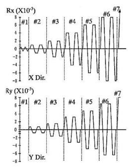
Figure 2-15 Loading Cycle Schematics for Multi-axis Cyclic Tests
