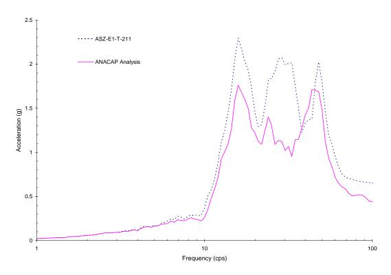
Figure 5-24 Comparison of Z-Direction Response between ANACAP Analysis at Upper Slab Corner No.2 and Measured Result for Run-2'
