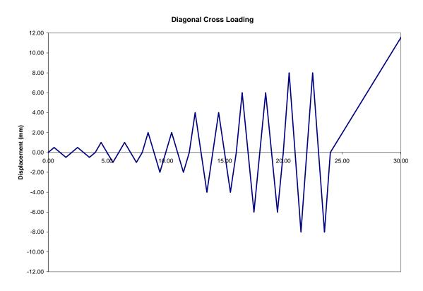
Figure 4-3 1-D Displacement Loading Pattern
