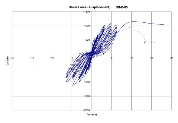
Figure 4-34 Qy – Dy Relation for Diagonal Cross Loading
