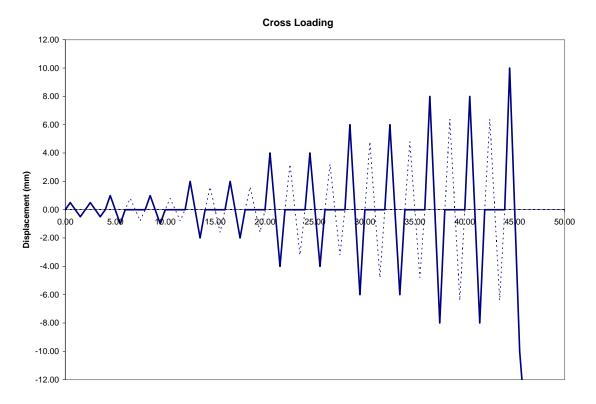
Figure 4-6 Cross Displacement Loading Pattern
