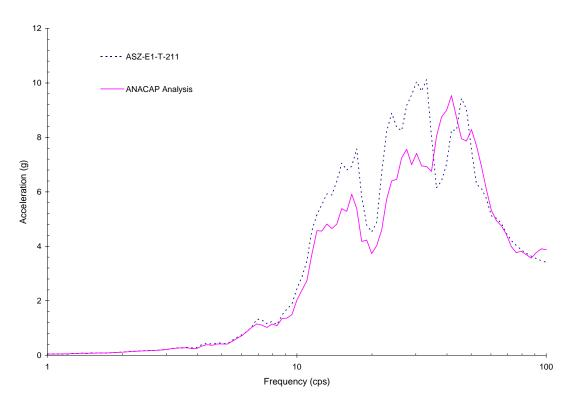
Figure 5-51 Comparison of Z-Direction Response between ANACAP Analysis at Upper Slab Corner No.2 and Measured Result for Run-4
