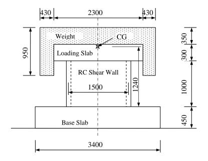
Figure 5-1 Elevation of DT-B-02 Model (Unit: mm)
