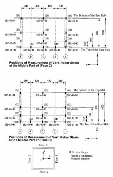
Figure 2-26 Schematic Locations of Strain Gauges of Vertical Rebars of Walls (C & D)
