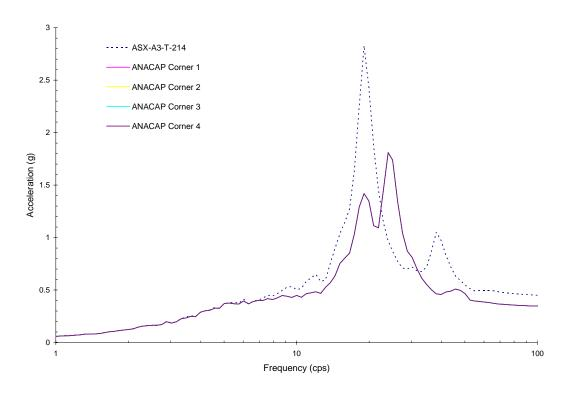
Figure 5-9 Comparison of X-Direction Response between ANACAP Analysis at Upper Corners of Shear Walls and Measured Data for Run-1
