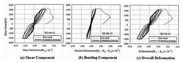
Figure 2-32 Comparison of JEAG Calculations of Hysteresis Loops with Test Data
