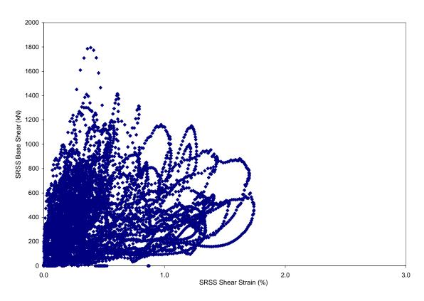
Figure 5-83 ANACAP Calculated SRSS Base Shear vs. SRSS Shear Strain without Considering Prior Damages for Run-6
