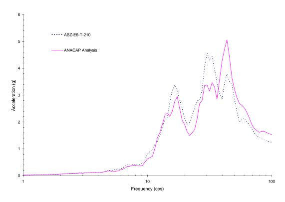
Figure 5-34 Comparison of Z-Direction Response between ANACAP Analysis at Upper Slab Corner No.3 and Measured Result for Run-3
