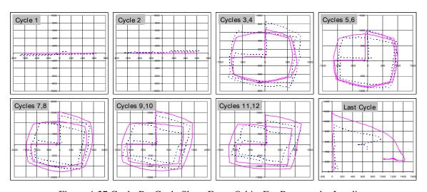
Figure 4-27 Cycle-By-Cycle Shear Force Orbits For Rectangular Loading
