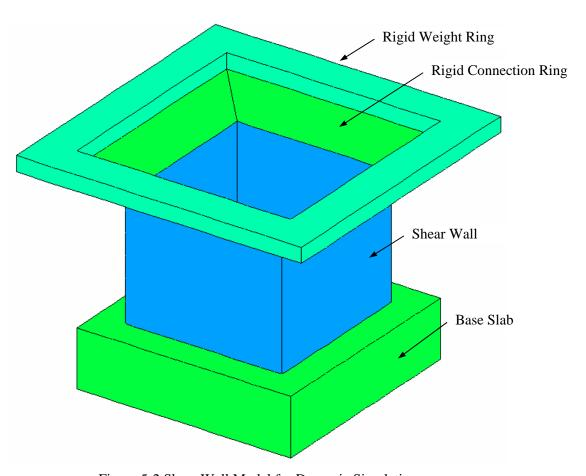
Figure 5-2 Shear Wall Model for Dynamic Simulation
