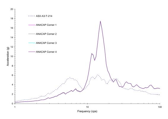
Figure 5-85 Comparison of X-Direction Response from ANACAP Analysis Considering No Prior Damages but with X-Input Motion only and Test Result for Run-6
