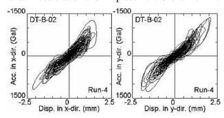
Figure 2-47 Horizontal Hysteresis Loops from Run 4 for DT-B-02
