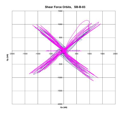
Figure 4-37 Shear Force Orbits for Diagonal Cross Loading
