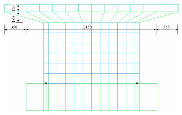
Figure 5-4 Shear Wall Mesh for Dynamic Simulation (Elevation, Unit mm)
