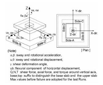
Figure 2-39 Schematic Notations employed in Displays of Shaking Table Test Results
