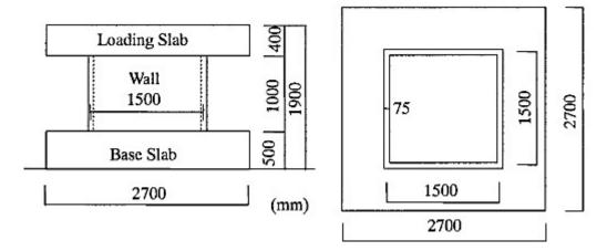
Figure 2-3 Box-Type Shear Wall Specimen for Multi-axis Cyclic Tests
