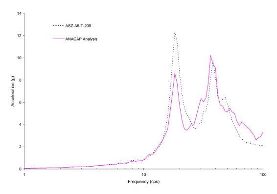
Figure 5-20 Comparison of Z-Direction Response between ANACAP Analysis at Upper Slab Corner No.4 and Measured Result for Run-2
