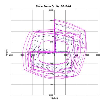
Figure 4-26 Shear Force Orbits for Rectangular Loading
