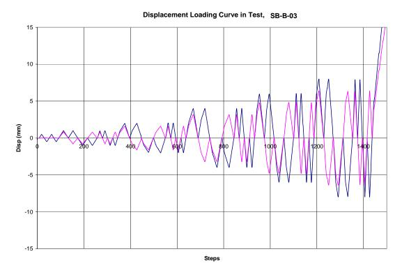
Figure 4-12 Displacement History at the Top of Shear Wall for SB-B-03
