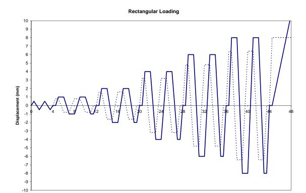
Figure 4-4 Rectangular Displacement Loading Pattern
