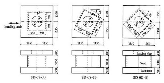
Figure 2-1 Uni-Directional Cyclic Test specimens (SD-08 Series)
