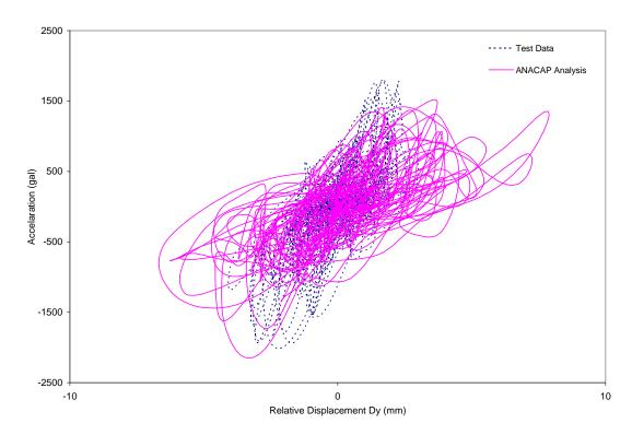
Figure 5-82 Comparison of ANACAP Hysteresis Loop without Considering Prior Damages for Run-6 in Y-Direction and Test Result
