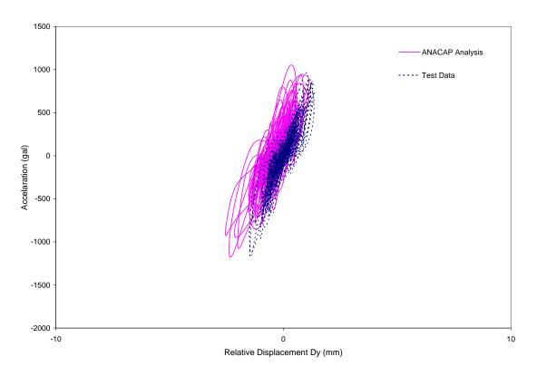
Figure 5-46 Comparison of Hysteresis Loops in Y-Direction for Run-3'
