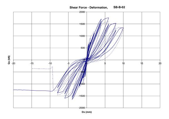
Figure 4-28 Qx – Dx Relation for Cross Loading
