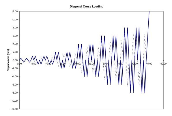
Figure 4-8 Diagonal Cross Displacement Loading Pattern
