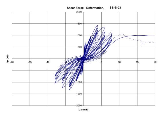
Figure 4-33 Qx – Dx Relation for Diagonal Cross Loading
