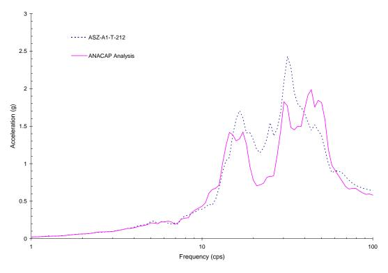
Figure 5-23 Comparison of Z-Direction Response between ANACAP Analysis at Upper Slab Corner No.1 and Measured Result for Run-2'
