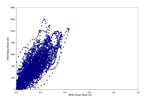
Figure 5-65 ANACAP Calculated SRSS Base Shear vs. SRSS Shear Strain for Run-5
