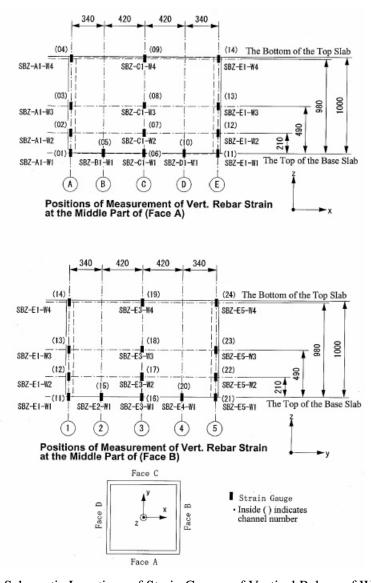
Figure 2-25 Schematic Locations of Strain Gauges of Vertical Rebars of Walls (A & B)
