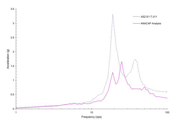
Figure 5-12 Comparison of Z-Direction Response between ANACAP Analysis at Upper Slab Corner No. 2 and Measured Result for Run-1
