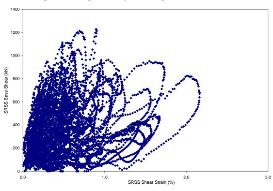
Figure 5-74 ANACAP Calculated SRSS Base Shear vs. SRSS Shear Strain for Run-6
