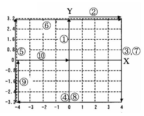
Figure 4-5 A Typical X-Y Displacement Orbit for Rectangular Loading [after Hiroshi, 2001]
