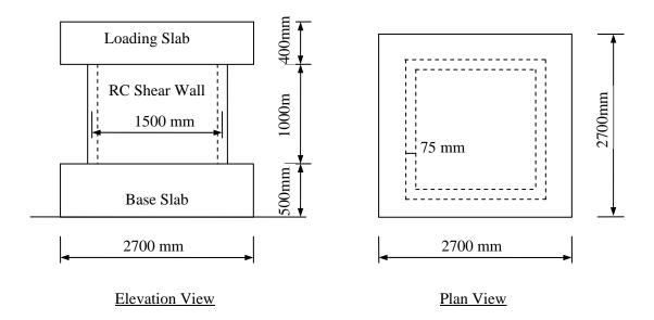
Figure 4-1 Box-shaped Shear Wall Dimension
