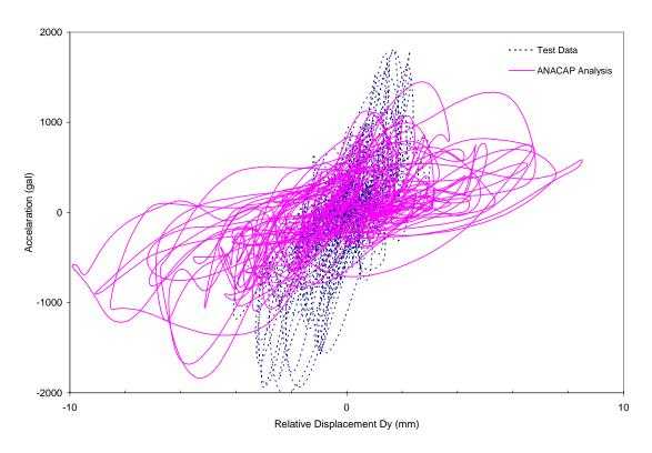
Figure 5-73 Comparison of Hysteresis Loops in Y-Direction for Run-6
