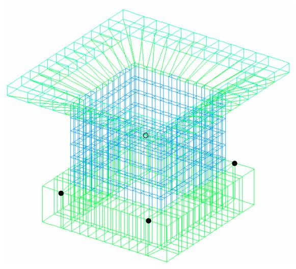
Figure 5-3 Shear Wall Mesh for Dynamic Simulation
