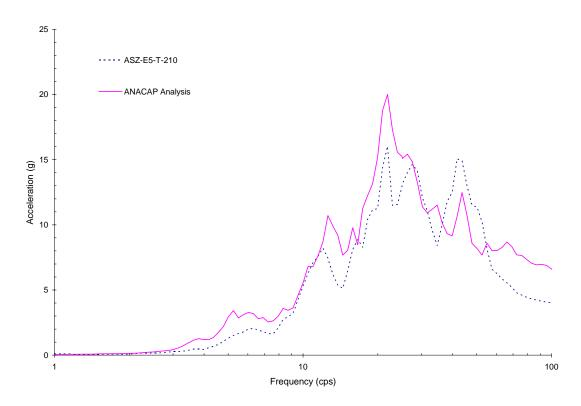
Figure 5-79 Comparison of ANACAP Analysis without Considering Prior Damages for Run-6 in Z-Direction at Upper Slab Corner No.3 and Measured Result
