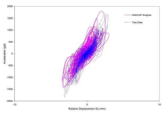
Figure 5-64 Comparison of Hysteresis Loops in Y-Direction for Run-5
