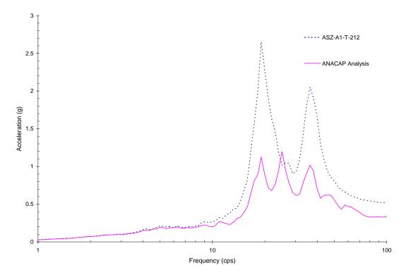
Figure 5-11 Comparison of Z-Direction Response between ANACAP Analysis at Upper Slab Corner No. 1 and Measured Result for Run-1
