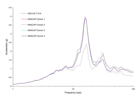
Figure 5-30 Comparison of X-Direction Response between ANACAP Analysis at Upper Corners of Shear Walls and Measured Data for Run-3
