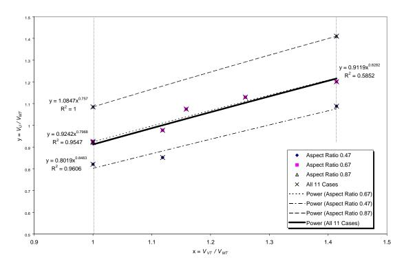
Figure 3-2 Regression Analysis of  $V_U/V_{MT}$  vs.  $V_{VT}/V_{MT}$
