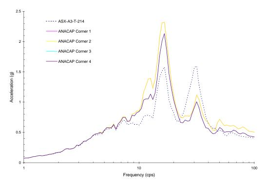
Figure 5-21 Comparison of X-Direction Response between ANACAP Analysis at Upper Corners of Shear Walls and Measured Data for Run-2'
