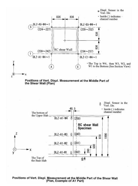
Figure 2-24 Schematic Locations of Displacement Gauges on Mid-Height of Walls
