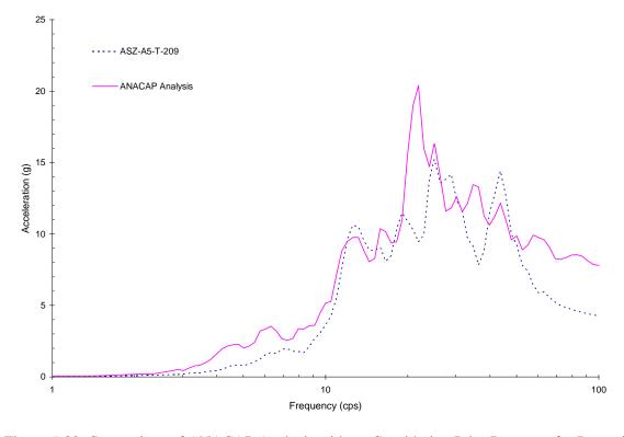
Figure 5-80 Comparison of ANACAP Analysis without Considering Prior Damages for Run-6 in Z-Direction at Upper Slab Corner No.4 and Measured Result
