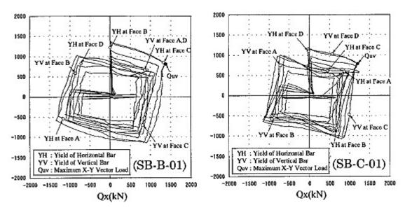
Figure 2-17 Computed Shear Force Orbits for Multi-Axis Tests
