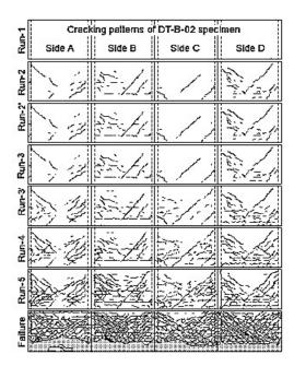
Figure 2-51 Progressive Development of Shear Wall Cracks for DT-B-02
