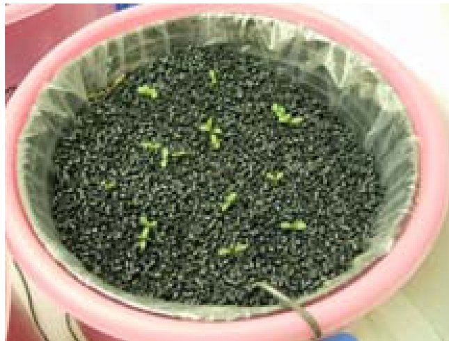
Figure 3.1. Hanford soil pot with germinating alfalfa showing secondary containment and plastic lined pot with polyethelene beads on top of soil and water sensor wire going into soil.
