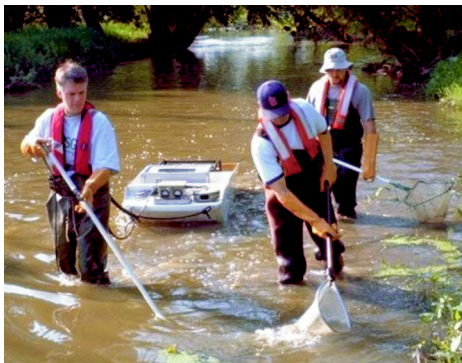
Figure 12. A barge-electroshocking unit being used to collect fish-community data.
