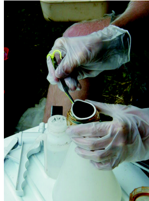
Figure 10. Filter used for periphyton chlorophyll- a , pheophytin- a , and ash-free dry mass determinations at Bassett Creek near Twin Lakes, Wisconsin.
