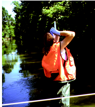
Figure 5. Measuring canopy cover from the center of the stream at Addison Creek at Bellwood, Illinois.
