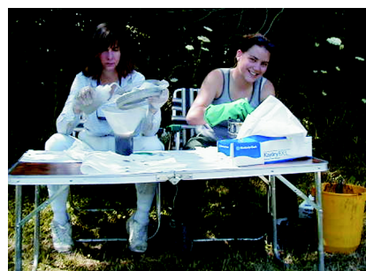
Figure 8. Sieving bed sediment for metal and particle size determination at Bassett Creek near Twin Lakes, Wisconsin.
