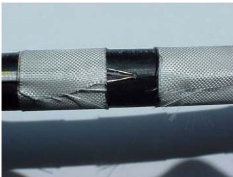
Figure 6-3: Photograph and schematic cutaway of a target cable instrumented with bare-bead type K thermocouples on the surface and just under the outer insulation.
