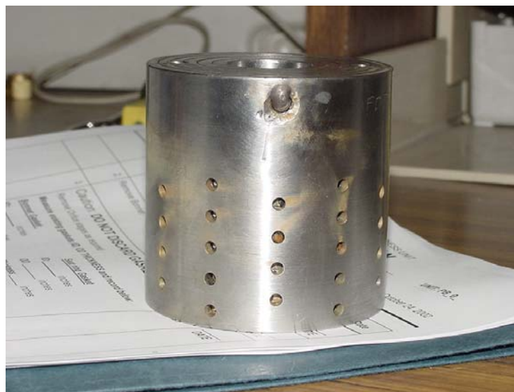
Figure 2. Recirculation Flow Restricting Orifice
