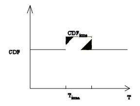
Figure 1. The shadowed area is the additional risk caused by a safety significant system component unavailability. The annual indicator is the sum of all individual unavailabilities during the year.
