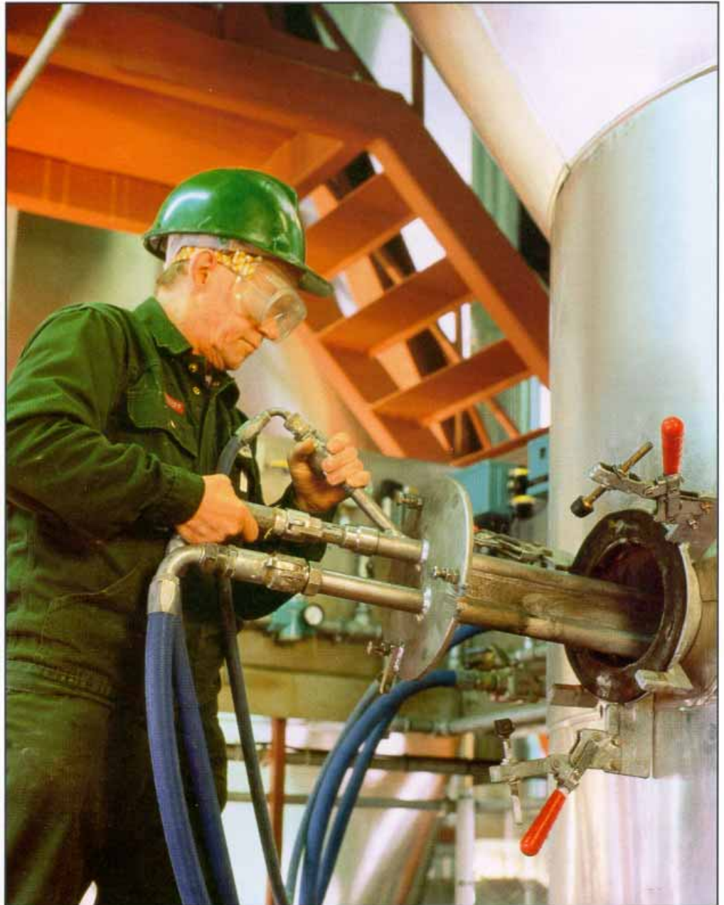
The GSA nozzle is easily removed for inspection and service.
