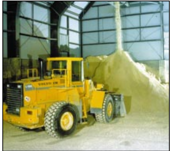
By-product gypsum storage prior to wallboard manufacture.
