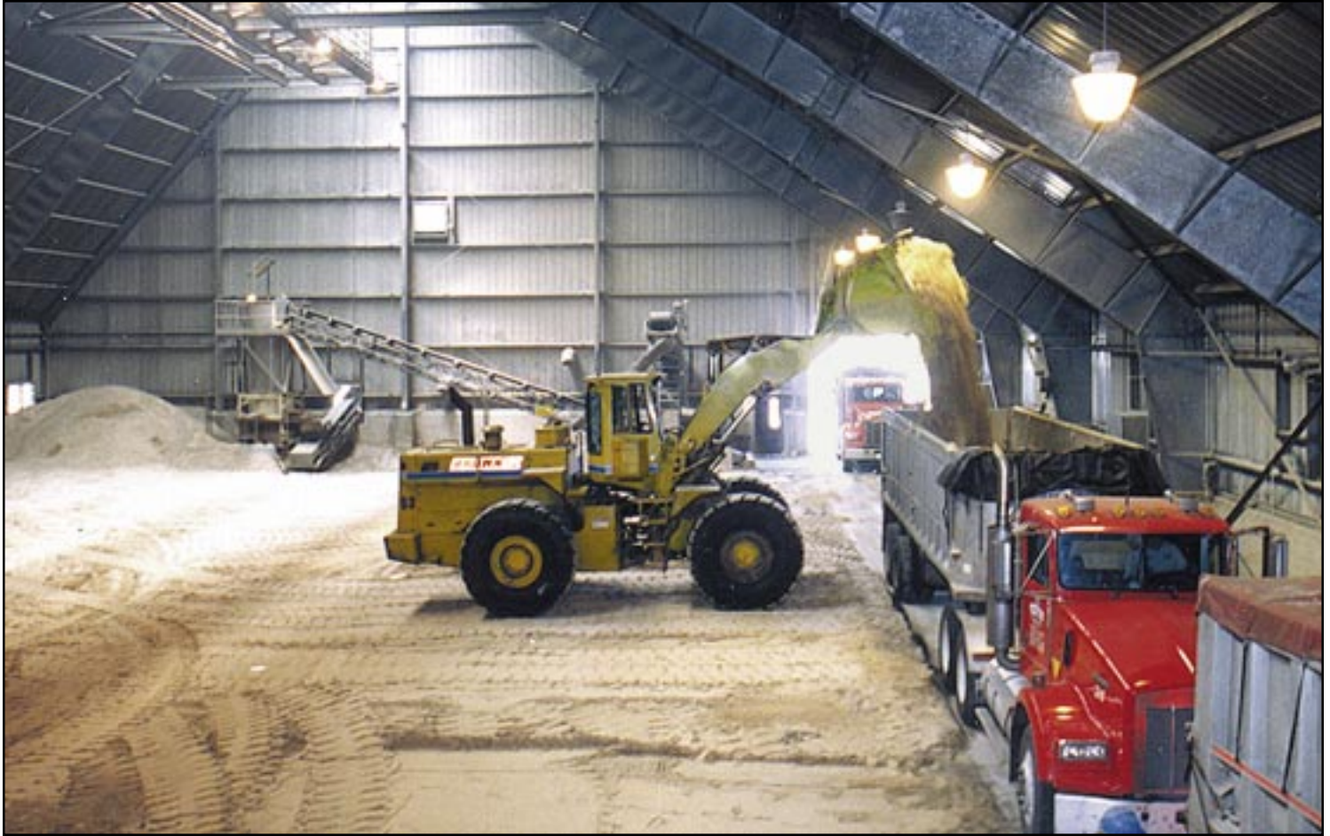
Loading FGD by-product gypsum for transport to wallboard plant.
