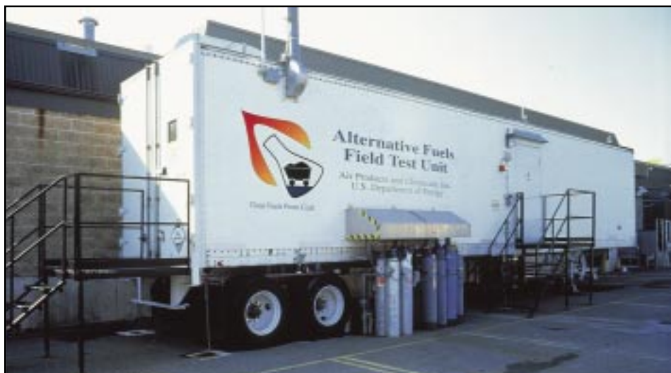
The Alternative Fuels Field Test Unit, containing state-of-the-art equipment, is used to determine the effect of poisons on catalyst performance and life.
