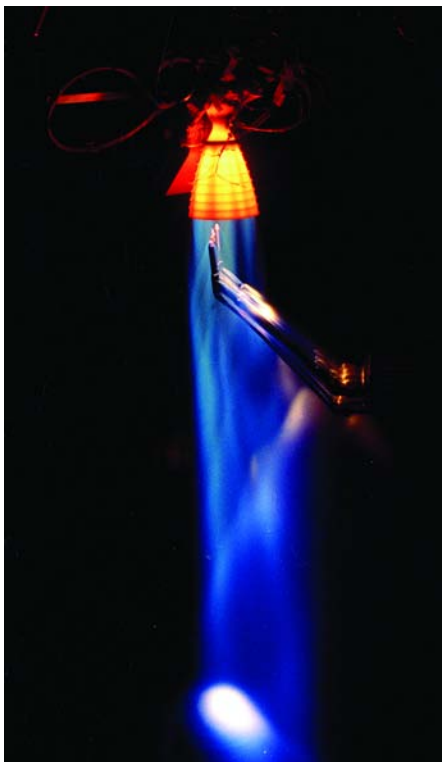
Water-cooled probes measure exhaust characteristics of 100 lbf attitude control thruster.
