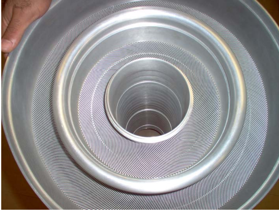
Figure 2: The core of HFIR, showing the inner (IFE) and outer (OFE) fuel elements.
