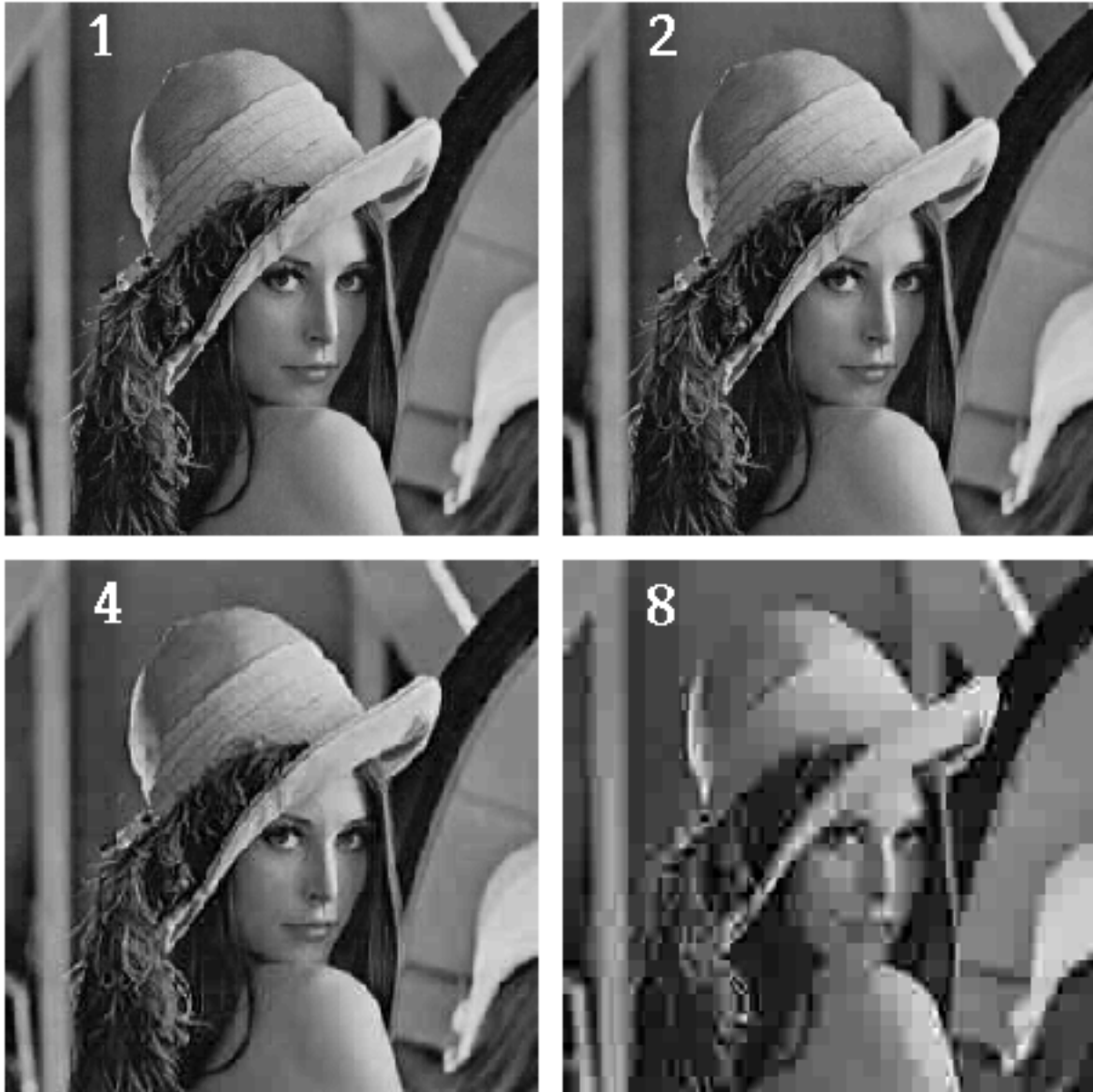
Figure 5. The Lena image compressed using custom matrices designed for perceptual error levels ( \Psi ) of 1, 2, 4, and 8. Corresponding bit rates were 2.28, 1.47, 0.72, 0.24. The original image had dimensions of {256,256}.
