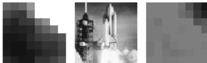
Figure 4. Iterative estimation of the custom quantization matrix \hat{q}_{ij} . The three panels in each row show quantization matrix q_{ij} , the reconstructed image using q_{ij} , and the perceptual error matrix p_{ij} . The labels indicate the iteration trial, the current JPEG bit-rate, and the maximum difference between p_{ij} and \Psi (discounting those for which the maximum error is always less than \Psi ). The image was \{64,64\} , target \Psi was 1. For q_{ij} and p_{ij} , the DC coefficient is at the lower left corner.
