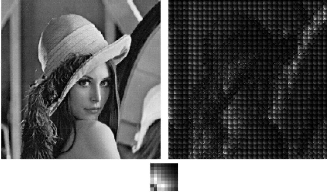
Figure 3. The Lena image and its masked sensitivity DCT ( m_{ijk}^{-1} ) for w_{ij}=0.7 and a_T=0.649 . If w_{ij}=0 and a_T=0 , all cells would be identical and would look like the inset ( 2 \times 2 ).
