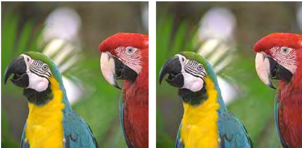
Figure 8. Image compressed with perceptually lossless DWT quantization matrix (left) and twice that matrix (right). Image dimensions are 256x256 pixels. Quantization matrix is designed for a viewing distance of 24 inches.
