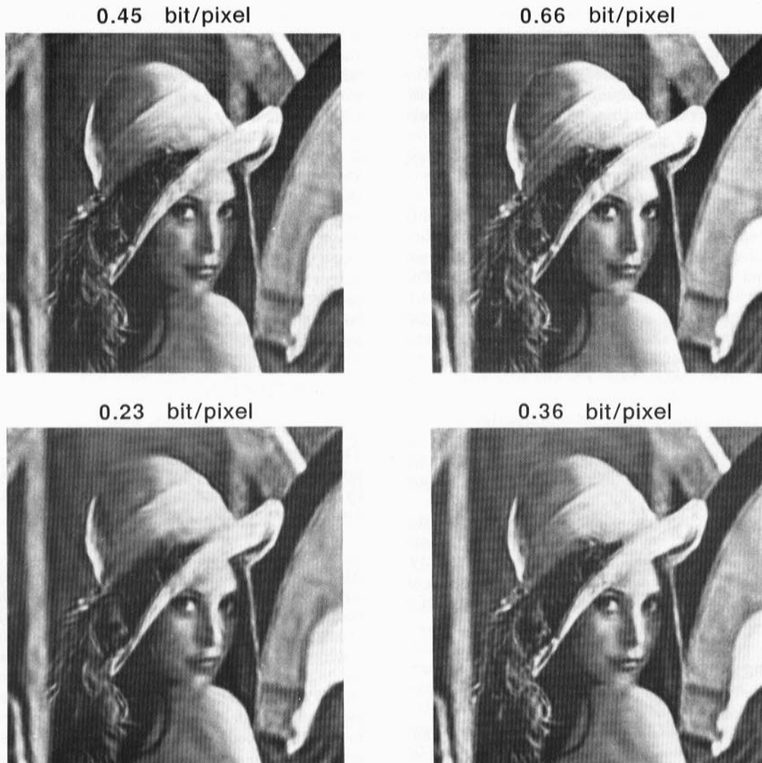
Fig. 19. Image of woman reconstructed from codes of various sizes. Entropies and Q at resolutions 5, 6, 7, and 8, respectively: 0.66 bit/pixel, 4, 3, 5, 7; 0.45 bit/pixel, 4, 5, 6, 7; 0.36 bit/pixel, 5, 4, 6, 8; 0.23 bit/pixel, 5, 5, 7, 8.
