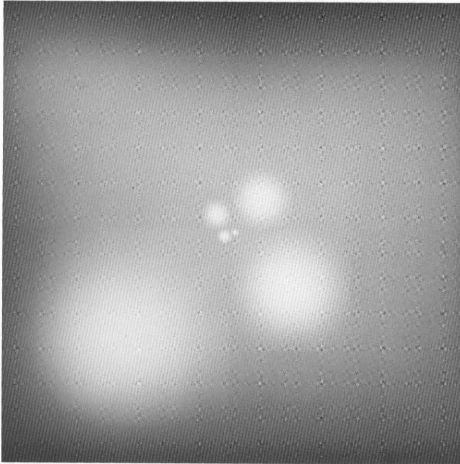
Fig.3. Fourier transforms of the set of basic sensors. Of the two Gaussians symmetrically placed about the origin, only one is shown. Axes are horizontal and vertical spatial frequency
