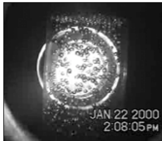
Hydrates, the small specks, have been formed in ESD's Sea-floor Process Simulator.
