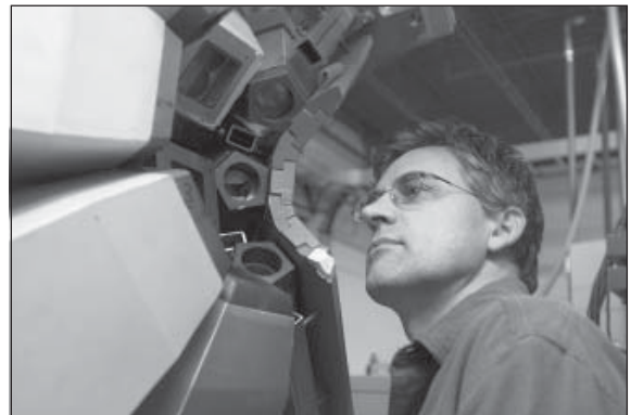
The Physics Division's David Radford examines a gamma-ray detector in the Holifield Radioactive Ion Beam Facility.
