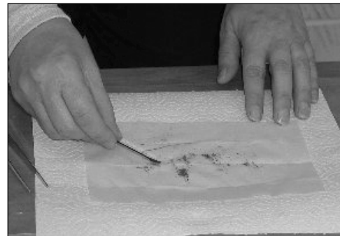
A technician for a lead-detection instrument vendor arranges particles on a dust-wipe sample.
