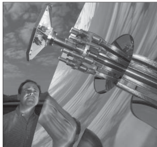
Jeff Muhs with a hybrid lighting system solar collector at the National Transportation Research Center.
