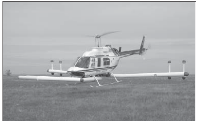
Flying close to the surface, helicopters equipped with the Oak Ridge Airborne Geophysical System can locate unexploded ordnance and other hazards hidden beneath the surface.
