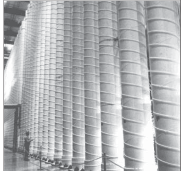
A gas centrifuge cascade at the former K-25 Site shows that the technology works on a grand scale.
