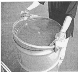
# 7 - Expanded ring being placed on Drum
