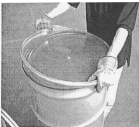
# 7 - Expanded ring being placed on Drum
