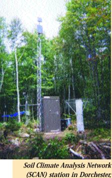
Son Chimate Analysis Network (SCAN) station in Dorchester, New Hampshire. This facility collects real time weather and snow pack data along with soil moisture, temperature and other soil temporal properties.
