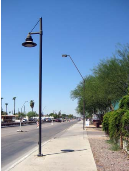
Pedestrian-scaled street lighting, in the foreground, contrasts with auto-oriented “cobra-head” lighting in the background.
