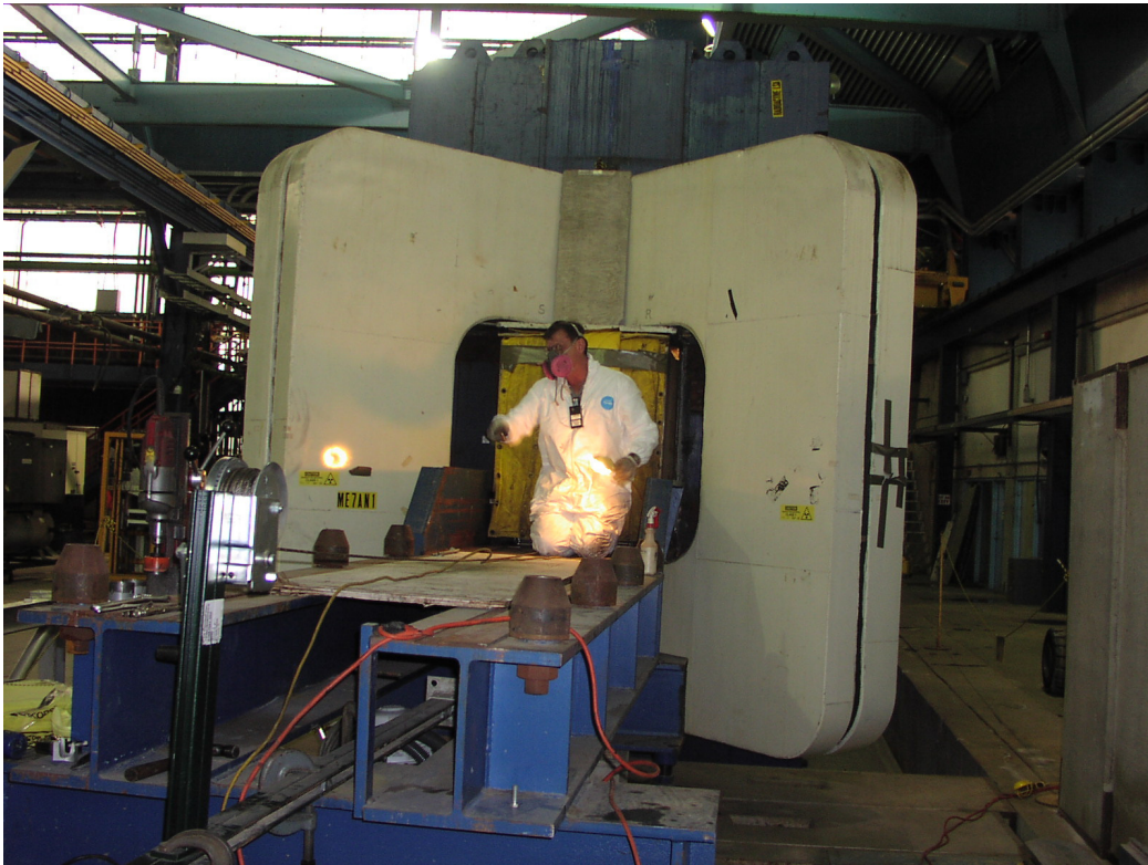
Worker Coming Out of Shielding Fixture within SM12 Magnet Beam Cavity
