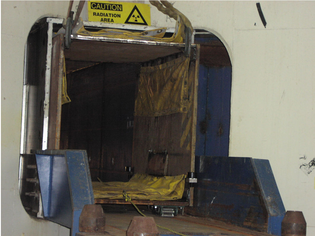
Shielding Fixture Inside SM12 Magnet Beam Cavity
