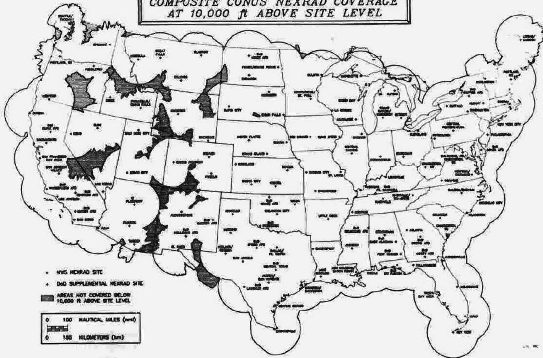
Fig. 1. WSR-88D network coverage at 10 000 ft (3.05 km) above site level for the contiguous United States. Hatched regions represent
