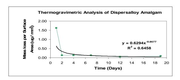
Note difference in scale: high-Cu alloy releases significantly more Hg than "oldfashioned" low-Cu alloy
