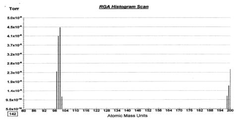
The RGA analysis reveals that only mercury is present in the emitted vapor, and it exactly matches the signature of pure mercury (one line for each isotope, for ions of +1 and +2 charge) in the mass spectrometer
