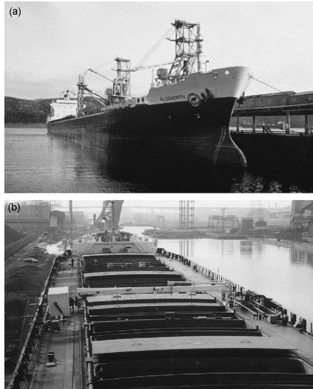
Fig. 1. (a) The MV Algonorth , a Seaway-sized dry bulk carrier used to evaluate the biological effectiveness of a deck-mounted ABSF ballast water treatment system with nominal filtration options of 25, 50 and 100 \mu\text{m} . (b) Overview of the deck-mounted ABSF ballast water treatment system used evaluated onboard the MV Algonorth , a Seaway-sized dry bulk carrier.
