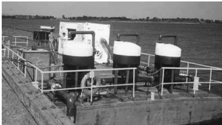
Fig. 2. The barge platform, moored in the Duluth-Superior Harbor of Lake Superior, used to evaluate the biological effectiveness of an ABSF ballast water treatment system with nominal filtration options of 25 or 50 \mu\text{m} .
