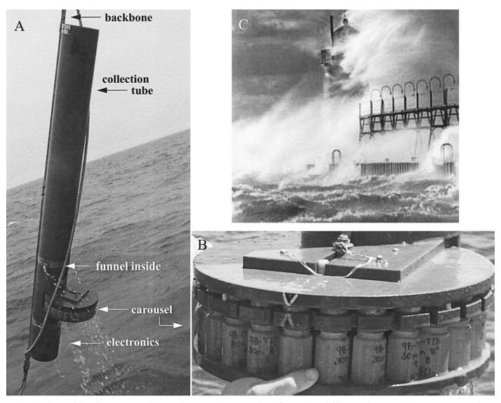
Fig. 1. Sequential sediment traps and the environment: (A) trap retrieval from Lake Michigan, noting essential components; (B) closeup of carousel, showing labeled 60-ml Nalgene collection bottles; (C) winter storm impacting harbor entry, South Haven, Michigan (courtesy Muskegon Chronicle).
