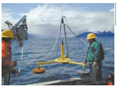
Installing the hydrophone, mounted on its customized aluminum anchor, near the mouth of Glacier Bay. The hydrophone anchor sits on the sea floor at 30 meters deep and is connected by a five-mile cable to a listening station at Park headquarters.
