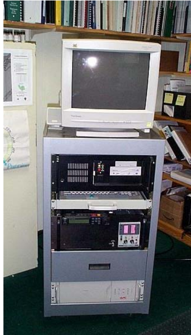
Fig. 3 Acoustic Data Acquisition System
