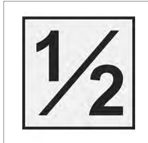
FIG ENR 5.7-1 Typical Runway Half-way Sign
