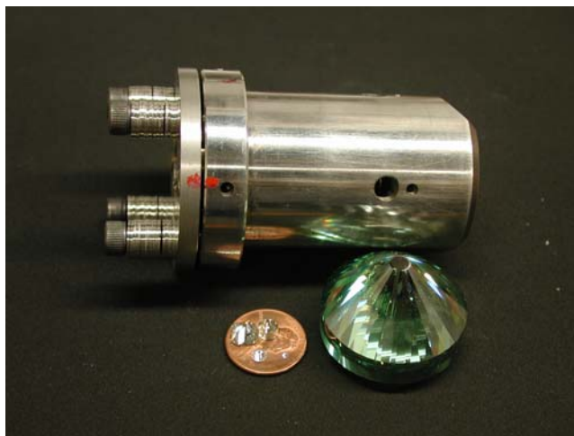
Figure 4.2.1 Megabar diamond anvil cell with natural diamonds sitting on the penny, and an anvil representative of the next generation of synthetic diamonds.
