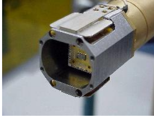
Figure 4.4.3 Prototype superconducting tunnel junction detector, which offers eV energy resolution and high count rate capability.
