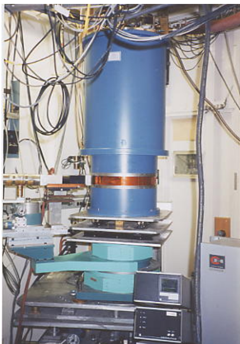
Figure 4.4.3 The superconducting magnet installed at X22B, NSLS. At NSLS-II, steady-state magnetic fields 20 T or more will be available on a beamline with more than two orders of magnitude more flux than at X22B, allowing entirely new classes of problems to be studied.
