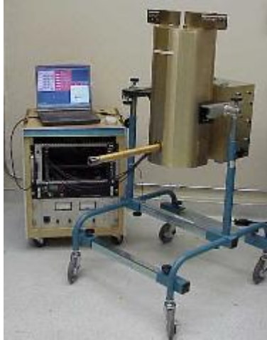
Figure 4.4.3 Prototype superconducting tunnel junction detector, which offers eV energy resolution and high count rate capability.
