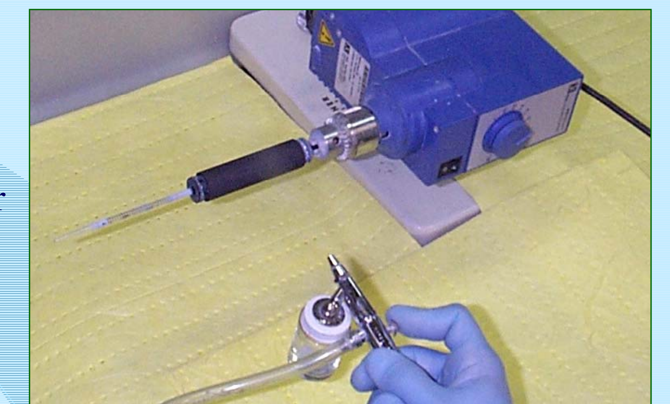
Demonstration of Laboratory Scale Coating Deposition on Cathode Support Tubes
