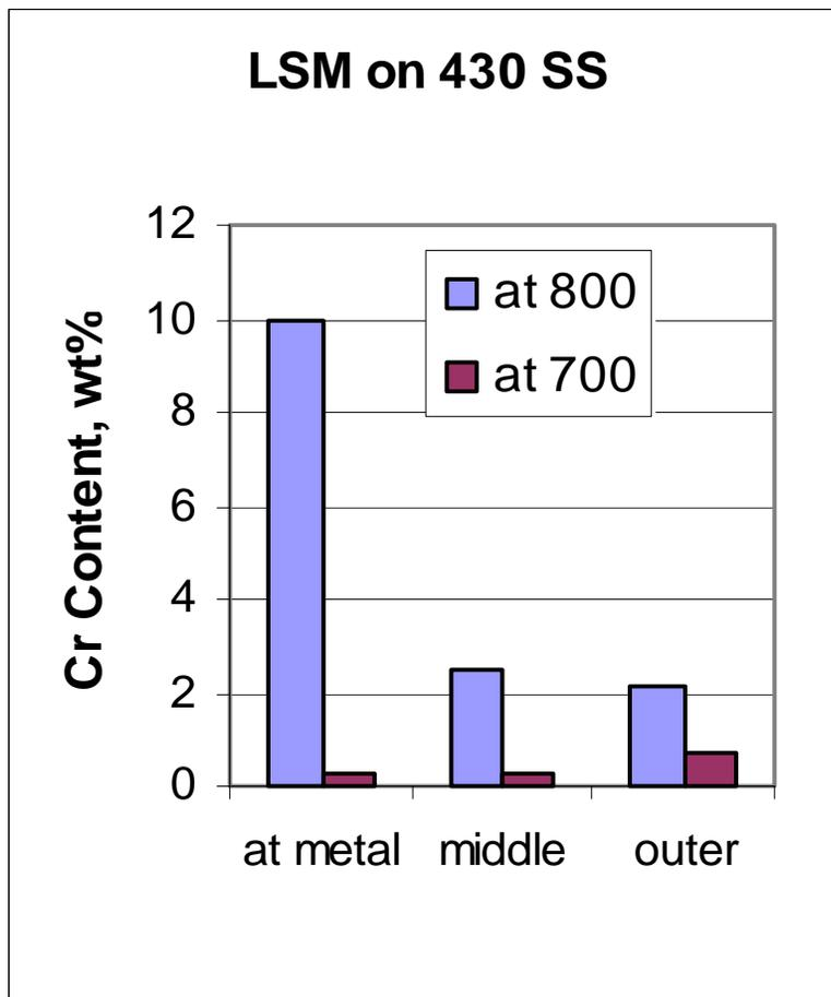
430 SS has a 1 micron chromia scale at 800°C and Cr depletion at 700°C, 10 micron Fe layer
