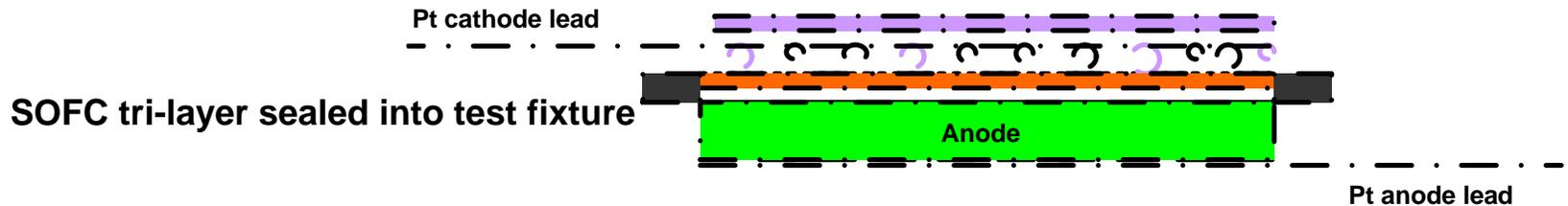
**Cross-section of SOFC Test Cell (6 cm<sup>2</sup>)**
