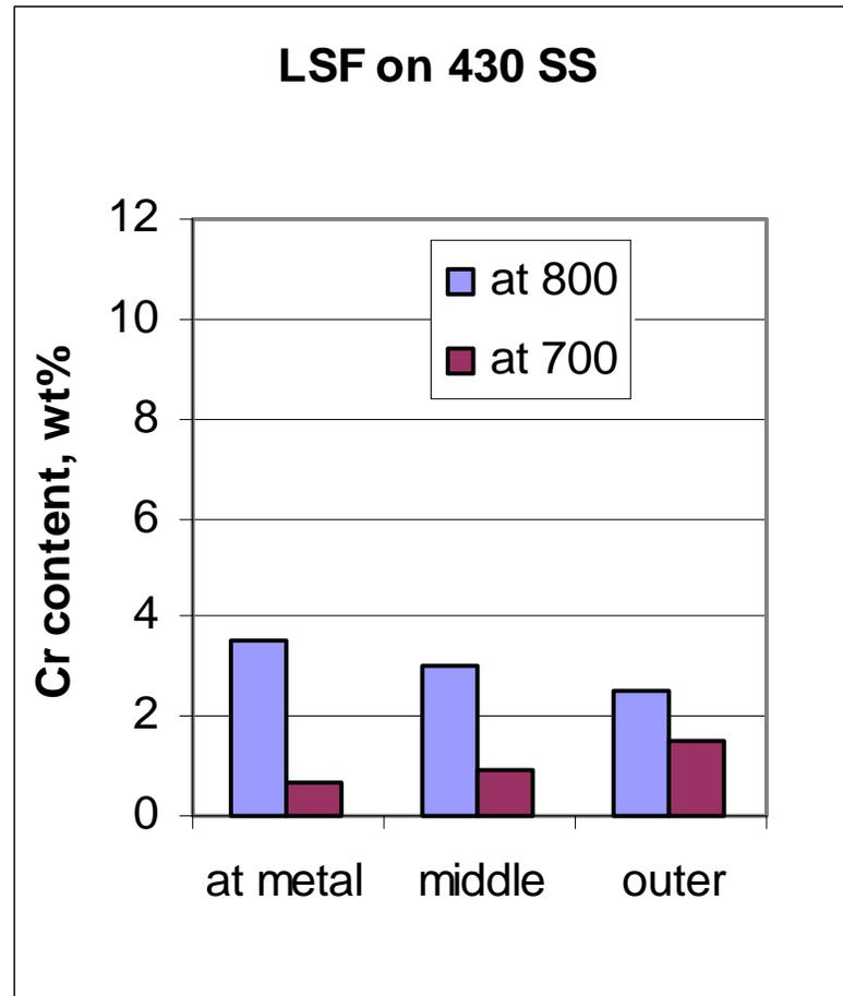
430 SS has a incomplete chromia scale at 800°C and Cr depletion at 700°C, 6-8 micron Fe layer
