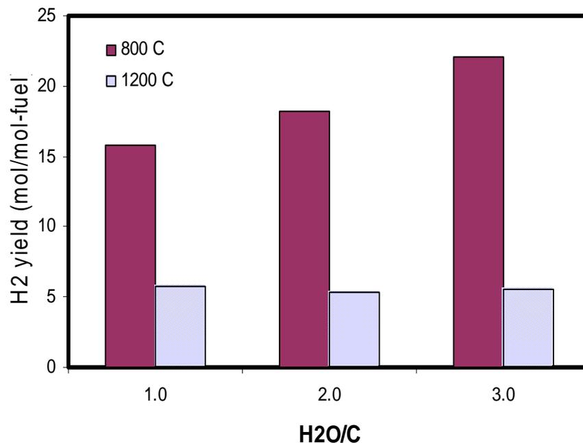
Optimizing calcination temperature resulted in significant activity improvement
