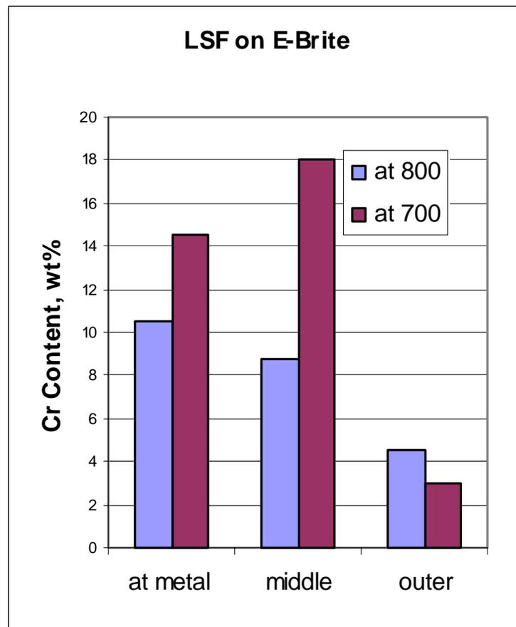
E-Brite chromia scale at 800C is 10 Micron vs. 1 micron at 700C
