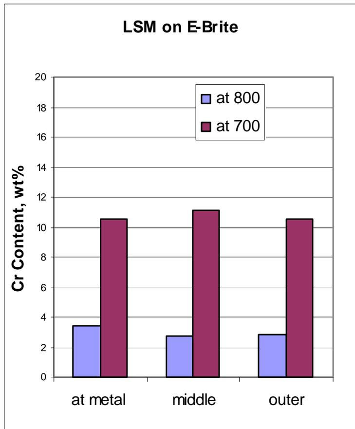
E-Brite chromia scale at 800C is 0.5 micron vs. 1 micron at 700C
