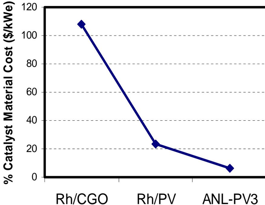
...while improved synthesis technique results in increase of reforming efficiency
