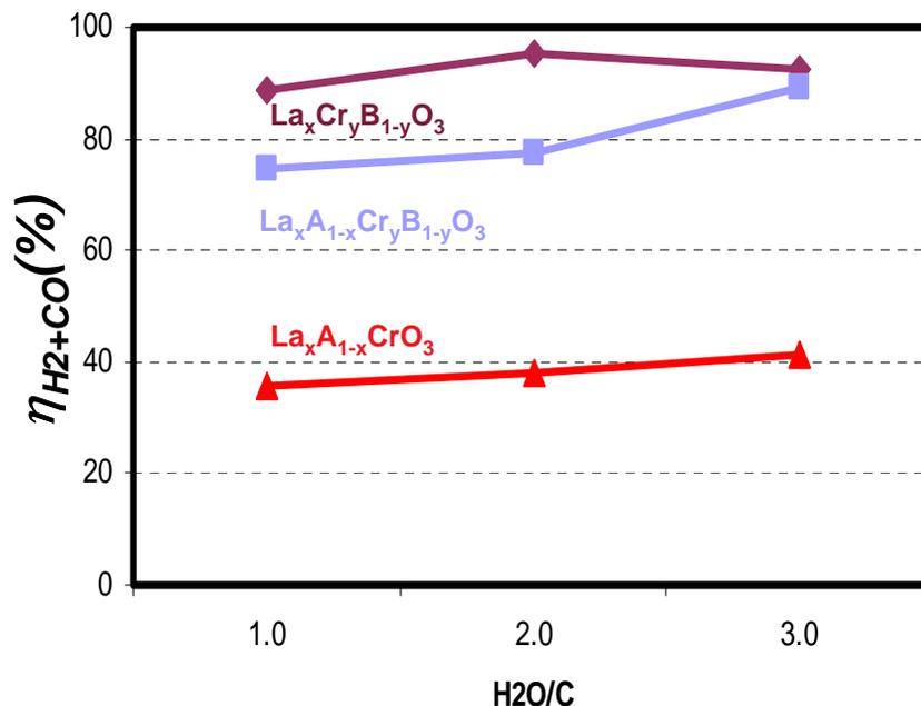
Cationic exchange at A & B sites can create lattice vacancy in perovskite structure and a better reforming catalyst
