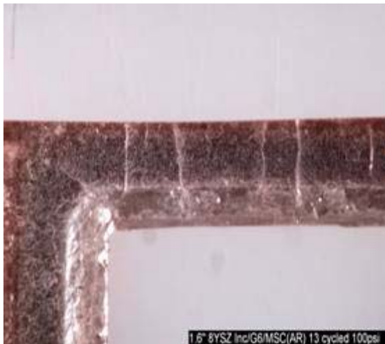
Muscovite mica degradation: wear particle through-thickness crack
