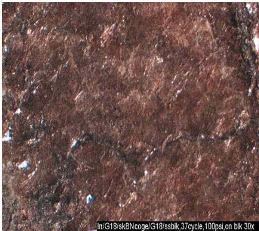
\text{Bi}_2\text{O}_3 after 37 cycles Inc/G18/mica/G18/SS430
