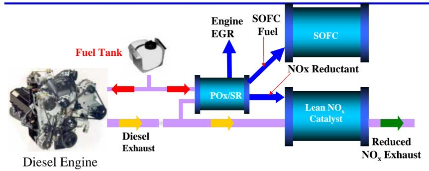
The reforming of diesel fuel potentially has simultaneous on-board vehicle applications:
