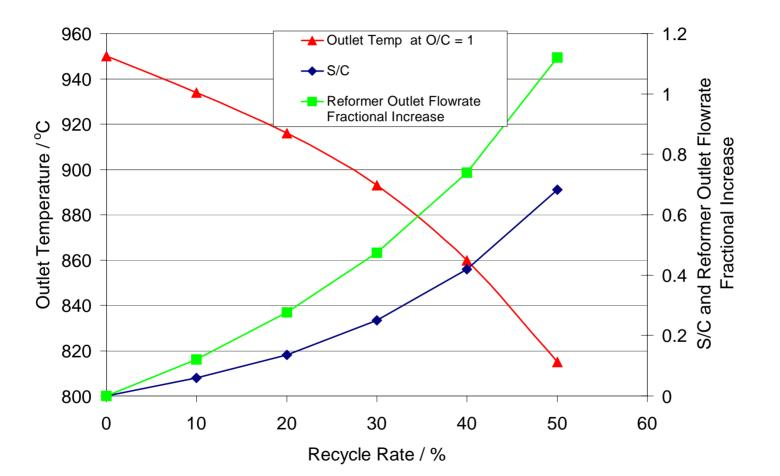
Green – Fractional increase in flow due to increasing gas volume due to recycle ratio, leads to larger reformer Fuel Cell Program – Los Alamos
