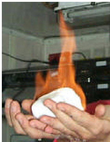
Gas hydrate is an ice-like substance composed of rigid cages of water molecules that enclose a low molecular weight gas—mainly methane (CH 4 )
