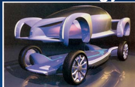
The AUTOnomi's control and propulsion system.
