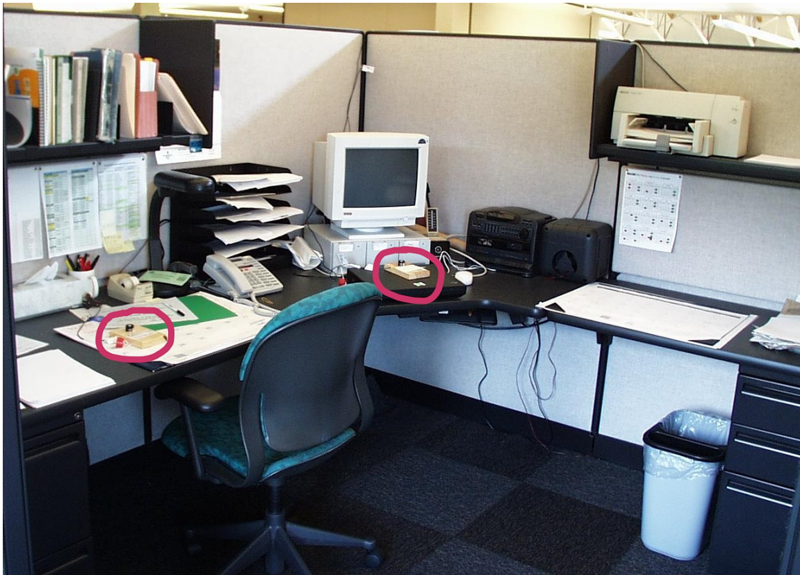
Figure 7-13 Placement of two photometers (shown circled) on the working plane of a cubicle
