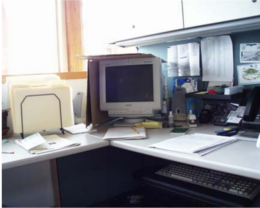
Figure 6-16 Glare problems caused by daylighting
