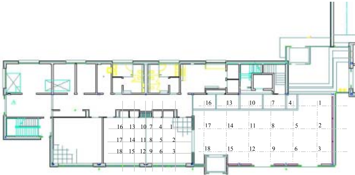
Figure 6-26 First-floor atrium and classroom handheld illuminance measurement locations
