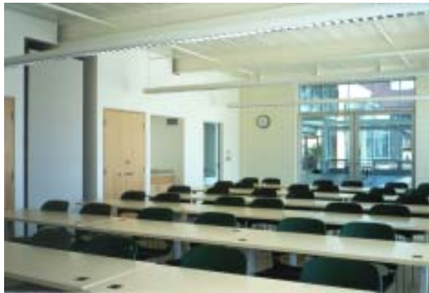
Figure D-11 First-floor classroom showing daylighting without electric lights
