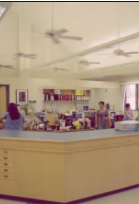
Photo: Architectural Energy Corporation Pearl Ridge Elementary School in Honolulu has no mechanical cooling system. It uses natural ventilation strategies. Ceiling fans and operable windows help keep the front office thermally comfortable.
