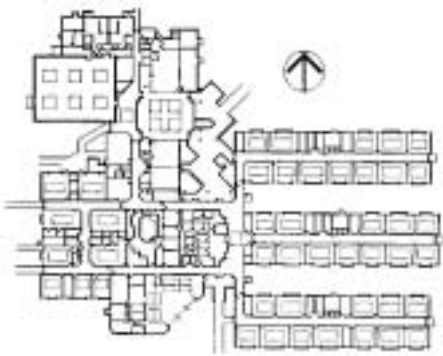
To optimize solar access, develop floor plan along an east-west axis.
