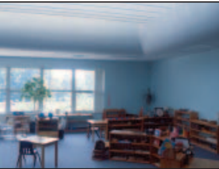
Light-colored interior finishes help the uniform distribution of natural light in the classroom.
