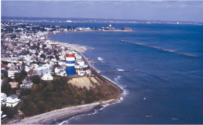
Figure 24. Stabilization of the eroding drumlins in Winthrop, Mass., cut off the supply of sediment to adjacent beaches. Seawalls, groins, and offshore detached segmented breakwaters are needed, along with occasional beach replenishment, to maintain the shoreline position.
