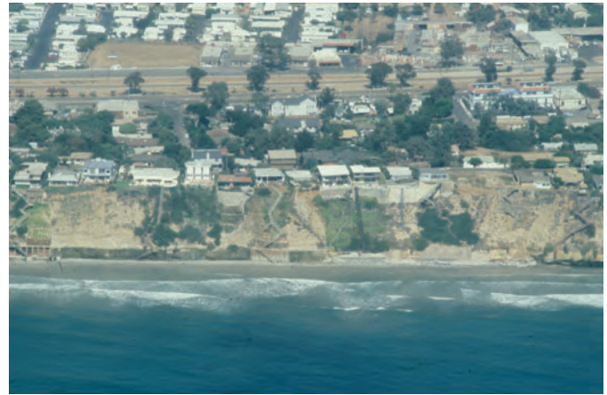
Figure 9. This nearly vertical coastal cliff in the Solana Beach area of southern California is fronted by a narrow beach and is under frequent attack by waves, which remove talus and erode the cliff base.
