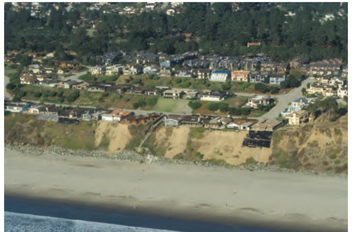
Figure 1. Developed sea cliffs in Northern Monterey Bay showing "riprap" at base of cliff and landslides from the 1989 Loma Prieta earthquake.
