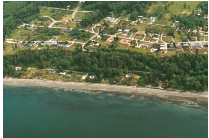
Figure 9. Large, prehistoric landslide on Whidbey Island. Portions of this slide periodically reactivate during wet weather. The toe of this landslide occurs slightly below beach level in this area. The landslide extends almost 2 km along the shoreline.
