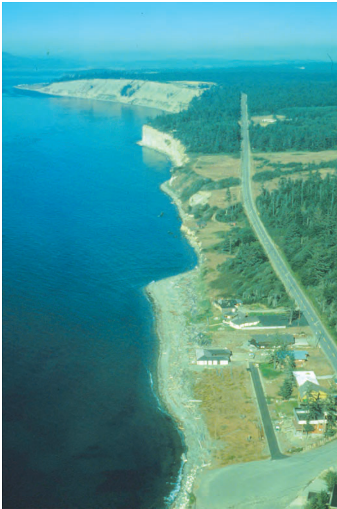
Figure 10. Irregular shoreline along western shore of Whidbey Island. Wave exposure is relatively uniform along this reach, and shape of shoreline is related to lithology and longshore redistribution of sediment by littoral processes. Beach in foreground is a barrier. Sharp point in mid-distance occurs where a resistant glacial till unit emerges at the toe of the bluff. (Photo by Gerald Thorsen).
