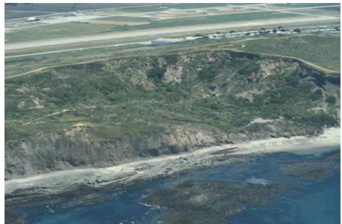
Figure 32. A large rotational slump in sedimentary rocks in the Half Moon Bay area of central California, showing a clearly developed rear scarp and undercliff (displaced landslide mass) with a cliff eroded at the seaward edge.
