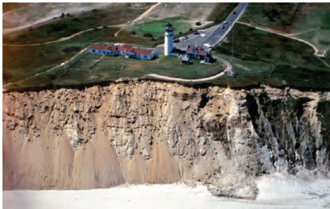
Figure 5. Highland Light on outer Cape Cod. Eroding bluff is mostly composed of outwash sand and gravel. The lighthouse was moved back from the bluff shortly after this photo was taken (photograph from James Allen, U. S. Geological Survey).
