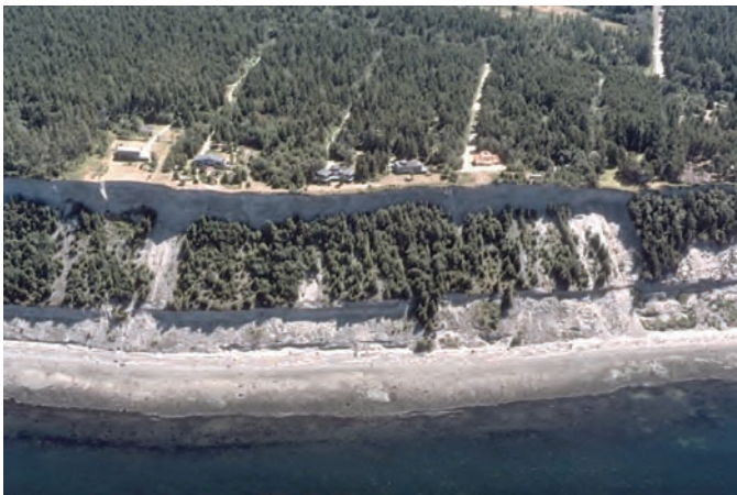
Figure 4. This 60-m-high bluff in Washington in glacial sediment shows the role of material composition in defining bluff shape. The upper till unit (in shade) fails in vertical slabs and does not support vegetation, whereas the central sandier outwash unit rests near the angle of repose, with substantial revegetation between erosional events. The lower, steep and unvegetated glacial unit is subject to wave action when storms and high tides coincide and when beach volume is reduced.
