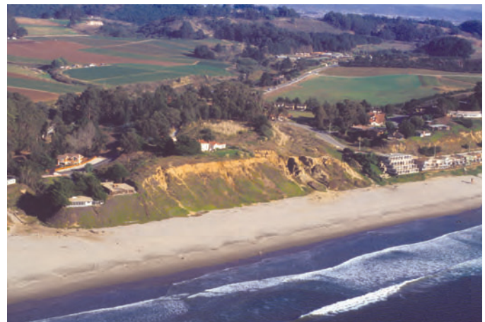
Figure 10. Coastal bluff with a convex profile in the northern Monterey Bay area of California, fronted by a wide protective beach. The convex profile exists because of a large talus build-up on the cliffs and reflects a dominance of terrestrial processes over wave erosion.
