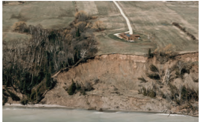
Figure 9. High (>30 m), complex bluff that failed in the early 1990s by a large deep-seated slump north of Milwaukee, Wisconsin, on the western shore of Lake Michigan.
