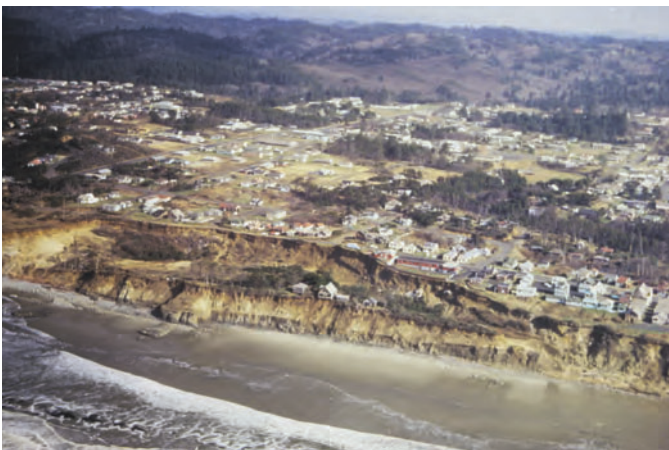
Figure 18. The 1942-43 landslide at Jump-Off Joe in Newport as photographed in 1961, with surviving houses on the slide block still inhabited. (Photo from the Lincoln County Historical Society, Newport.)
